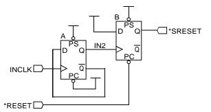
The circuit uses Flip-Flop A to delay the clock to Flip-Flop B. It divides INCLK, but that isn't important to the operation of the circuit. Depending on the circuitry used to generate a reset, a Schmidttrigger gate may be necessary. Using the specified min-max propagation delays, the delay characteristics of the circuit can be calculated.
