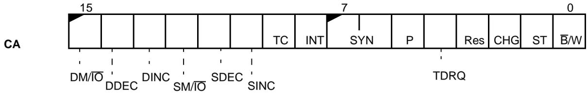
**DMA 0 Control Register (D0CON)**
