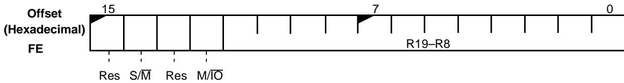
**Peripheral Control Block Relocation Register (RELREG)**
