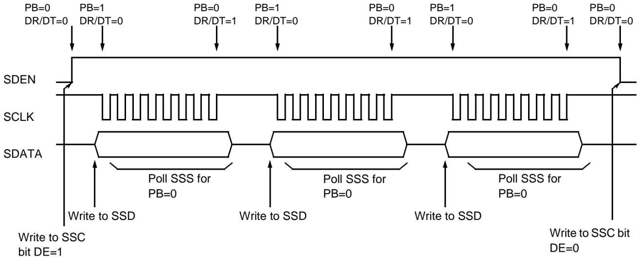
Figure 11-6 Synchronous Serial Interface Multiple Read
