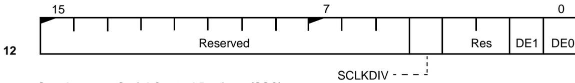
**Synchronous Serial Control Register (SSC)**
