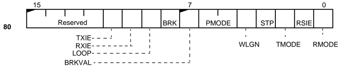
**Serial Port Control Register (SPCT)**
