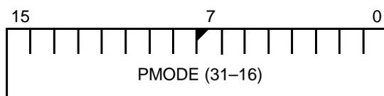
Figure 12-3 PIO Mode 0 Register (PIOMODE0, offset 70h)
