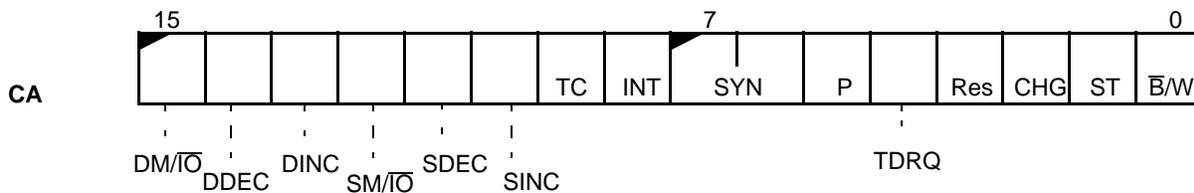
**DMA 1 Control Register (D1CON)**
