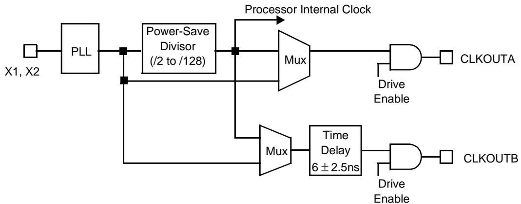
CLKOUTA and CLKOUTB operate at either the processor frequency or the PLL frequency. The output drivers for both clocks are individually programmable for drive enable or disable.
