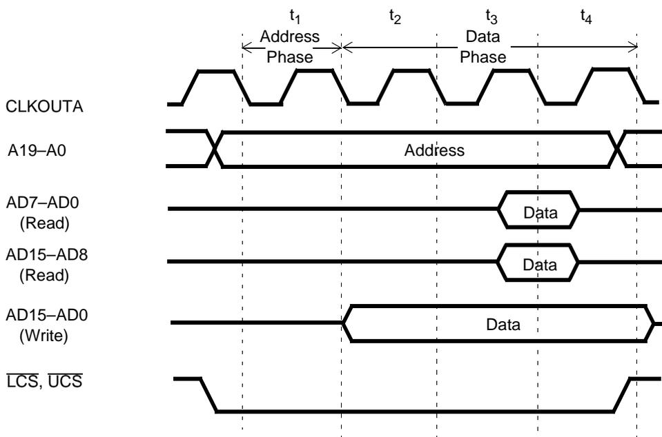
Figure 3-3 Am188EM Microcontroller Address Bus—Normal Read and Write Operation
