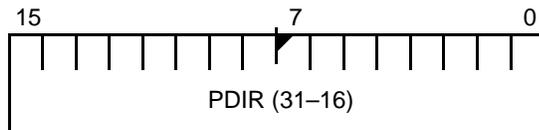
Figure 12-5 PIO Direction 0 Register (PDIR0, offset 72h)
