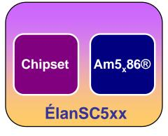
$Am5_x86$ ® core PCI bus SDRAM support  $AMDebug^{TM}$  technology
