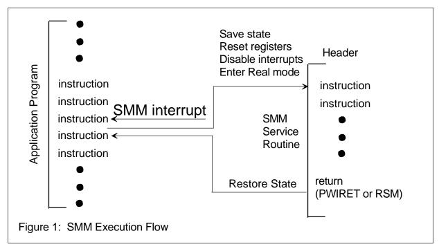
method uses standard interrupt protocol (assert INTR pin, execute power management routine, return via IRET instruction) and relies on the operating system to ensure proper operation. The traditional method is used today. The SMM method will be used in future systems.
