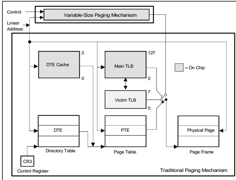
Figure 1-3. Paging Mechanism within the Memory Management Unit
