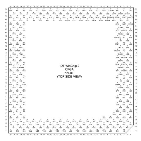
Figure 6-2. CPGA Pinout (Top Side View)
