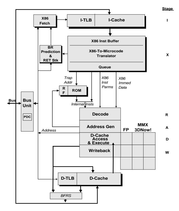
Figure 2-1. IDT WinChip 2 Processor Data Flow
