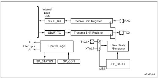
Figure 7-1. SIO Block Diagram
