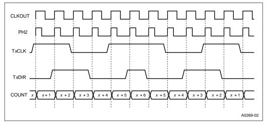
Figure 10-4. Quadrature Mode Timing and Count
