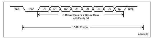
Figure 7-4. Serial Port Frames for Mode 1
