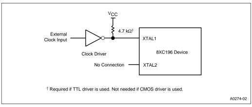
Figure 12-5. External Clock Connections
