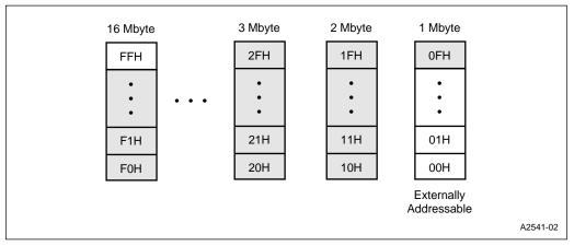
Figure 4-1. 16-Mbyte Address Space
