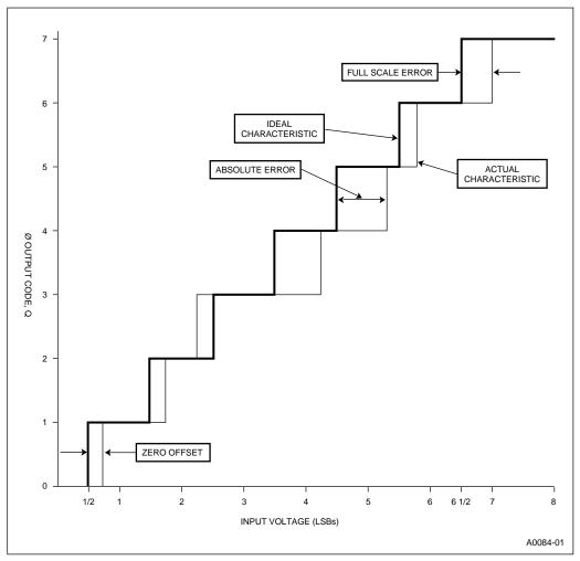
Figure 11-10. Actual and Ideal A/D Conversion Characteristics
