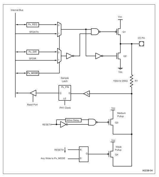
Figure 6-2. Bidirectional Port Structure
