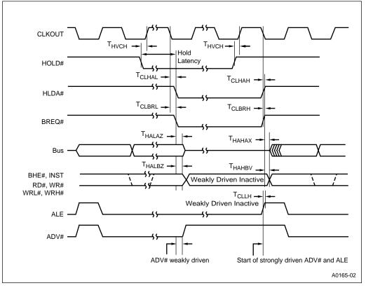
Figure 14-9. HOLD#, HLDA# Timing
