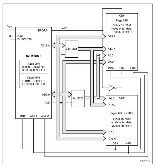
Figure 4-11. A 1-Mbyte System with a 16-bit Bus
