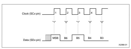
Figure 8-7. Variable-width MSB in SSIO Transmissions
