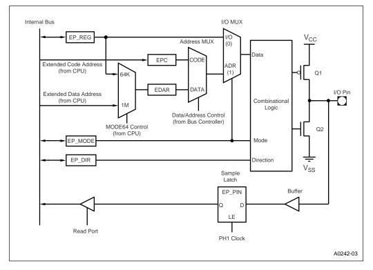
Figure 6-4. EPORT Block Diagram
