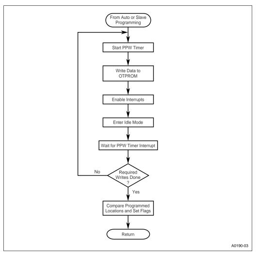
Figure 15-3. Modified Quick-pulse Algorithm
