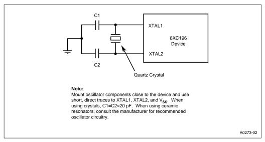
Figure 12-4. External Crystal Connections
