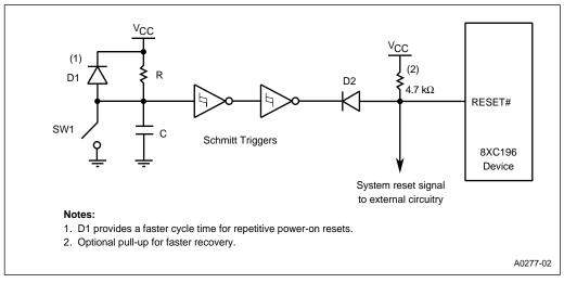
Figure 12-10. Example System Reset Circuit
