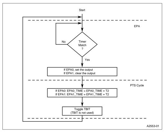
Figure 5-19. EPA and PTS Operations for the PWM Remap Mode Example
