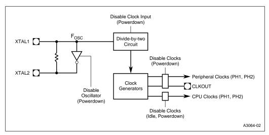
Figure 13-1. Clock Control During Power-saving Modes
