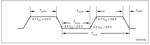
Figure 12-6. External Clock Drive Waveforms
