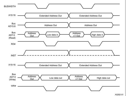
Figure 14-7. Timings for 8-bit Buses
