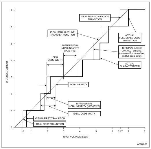
Figure 11-11. Terminal-based A/D Conversion Characteristic
