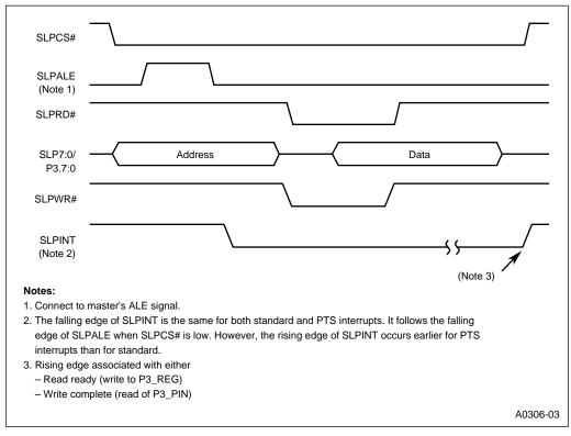
Figure 9-5. Standard or Shared Memory Mode Timings (Multiplexed Bus)
