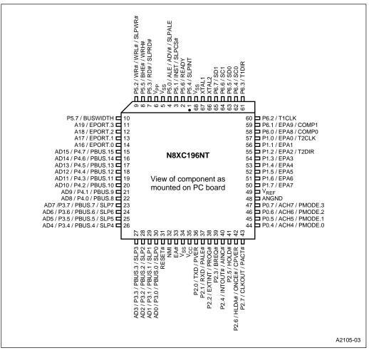
Figure B-1. 8XC196NT 68-lead PLCC Package
