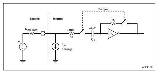
Figure 11-7. Idealized A/D Sampling Circuitry
