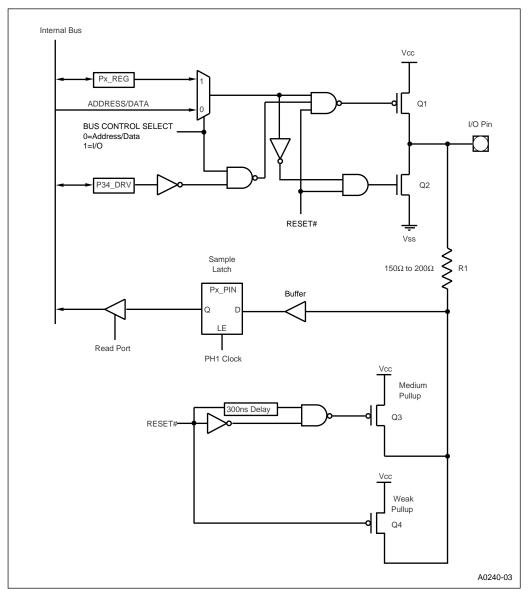
Figure 6-3. Address/Data Bus (Ports 3 and 4) Structure
