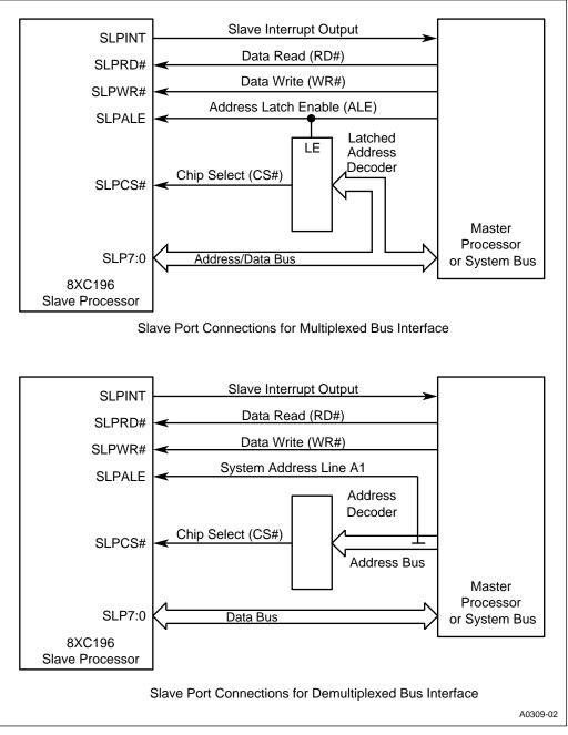
Figure 9-3. Master/Slave Hardware Connections
