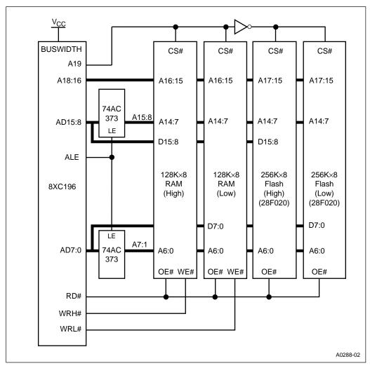
Figure 14-15. 16-bit System with Single-byte Writes to RAM
