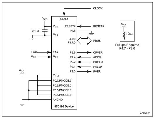
Figure 15-5. Slave Programming Circuit
