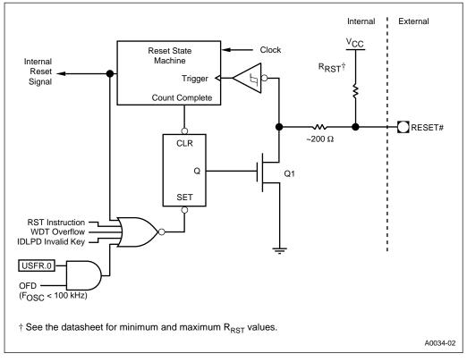
Figure 12-8. Internal Reset Circuitry
