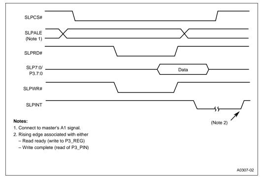
Figure 9-4. Standard Slave Mode Timings (Demultiplexed Bus)
