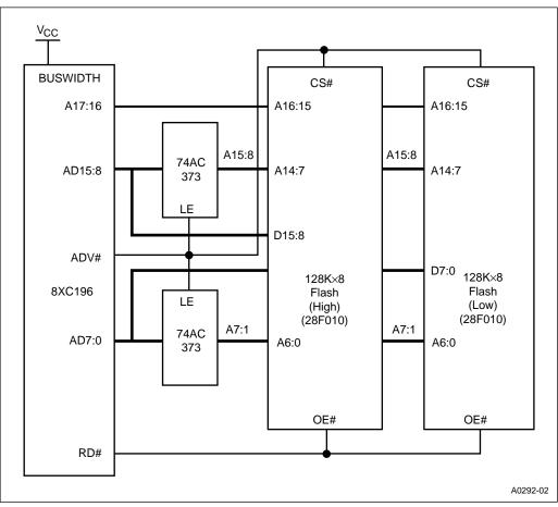
Figure 14-19. 16-bit System with Flash
