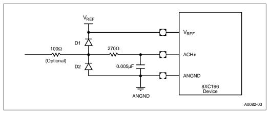
Figure 11-8. Suggested A/D Input Circuit
