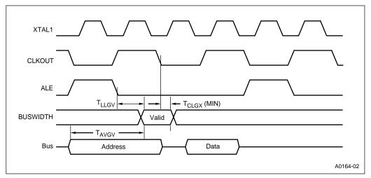
Figure 14-5. BUSWIDTH Timing Diagram
