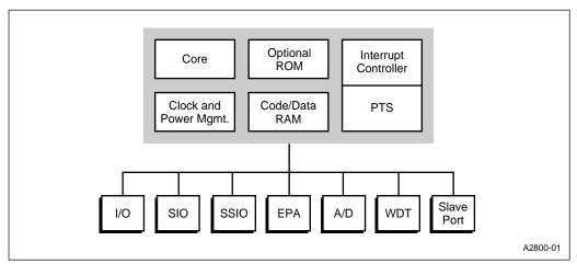
Figure 2-1. 8XC196NT Block Diagram
