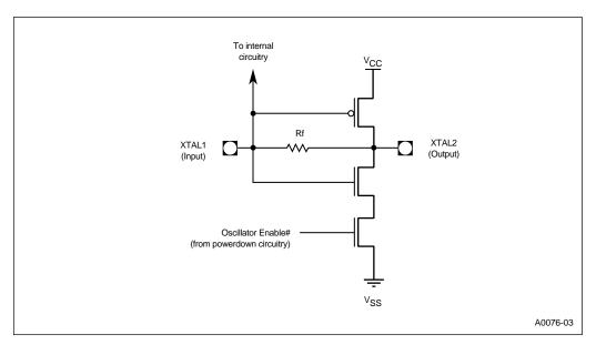
Figure 12-3. On-chip Oscillator Circuit
