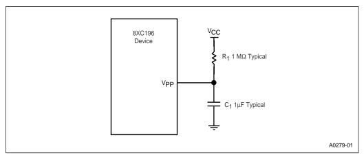
Figure 13-3. External RC Circuit
