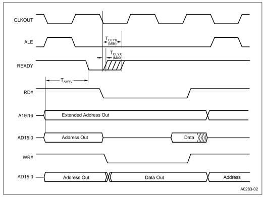
Figure 14-8. READY Timing Diagram
