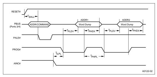
Figure 15-11. Dump Word Waveform
