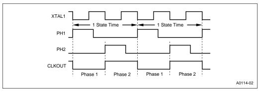
Figure 2-4. Internal Clock Phases
