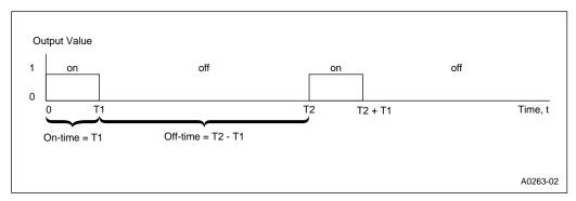
Figure 5-15. A Generic PWM Waveform
