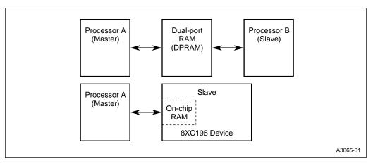
Figure 9-1. DPRAM vs Slave-port Solution
