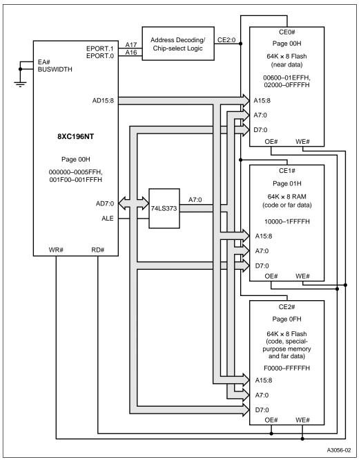
Figure 4-12. A 1-Mbyte System with an 8-bit Bus
