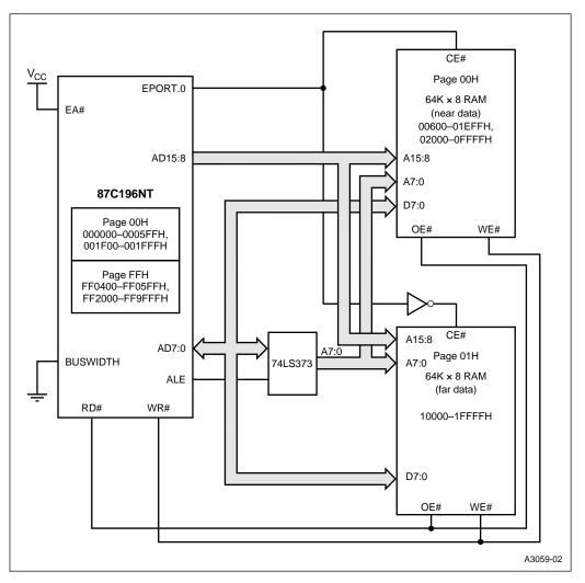
Figure 4-10. A 64-Kbyte System with Additional Data Storage
