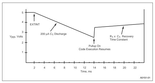
Figure 13-4. Typical Voltage on the V<sub>PP</sub> Pin While Exiting Powerdown
