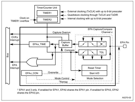
Figure 10-5. A Single EPA Capture/Compare Channel
