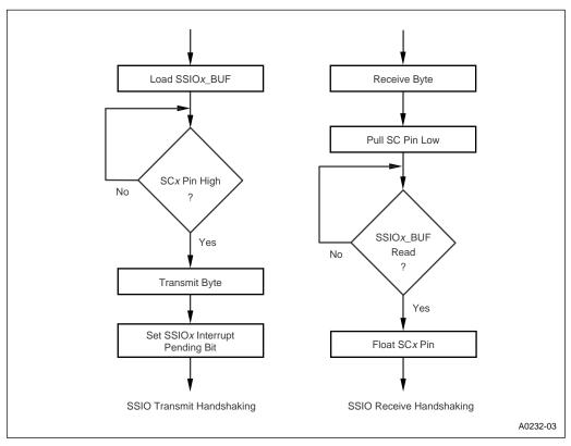
Figure 8-4. SSIO Handshaking Flow Diagram
