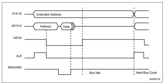
Figure 14-17. Comparison of ALE and ADV# Bus Cycles
