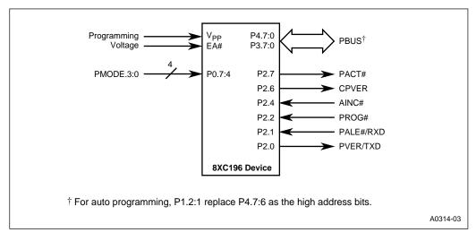
Figure 15-4. Pin Functions in Programming Modes
