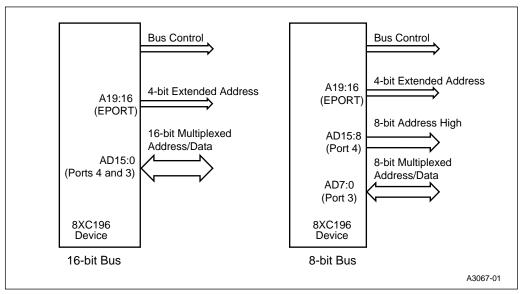
Figure 14-4. Multiplexing and Bus Width Options
