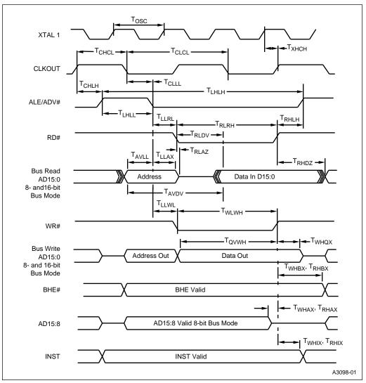
Figure 14-23. Mode 1 System Bus Timing
