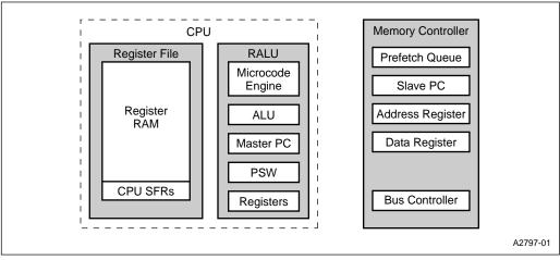
Figure 2-2. Block Diagram of the Core
