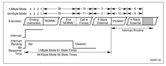
Figure 5-2. Standard Interrupt Response Time
