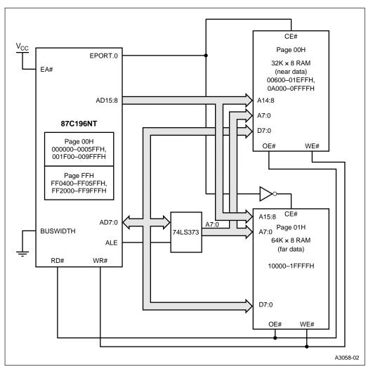
Figure 4-9. A 64-Kbyte System with an 8-bit Bus
