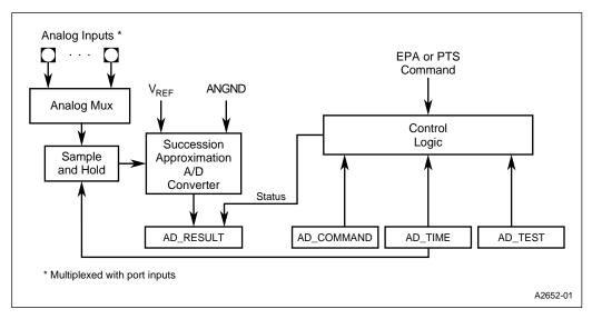
Figure 11-1. A/D Converter Block Diagram
