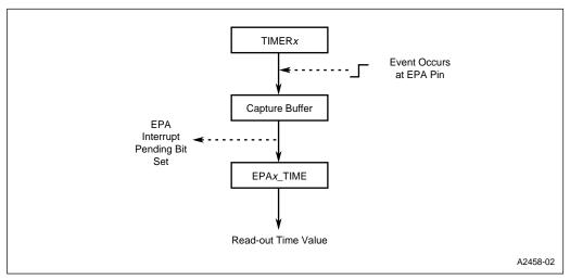
Figure 10-6. EPA Simplified Input-capture Structure
