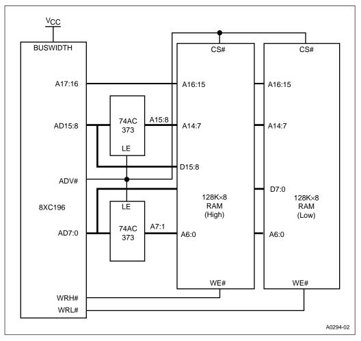
Figure 14-21. 16-bit System with RAM
