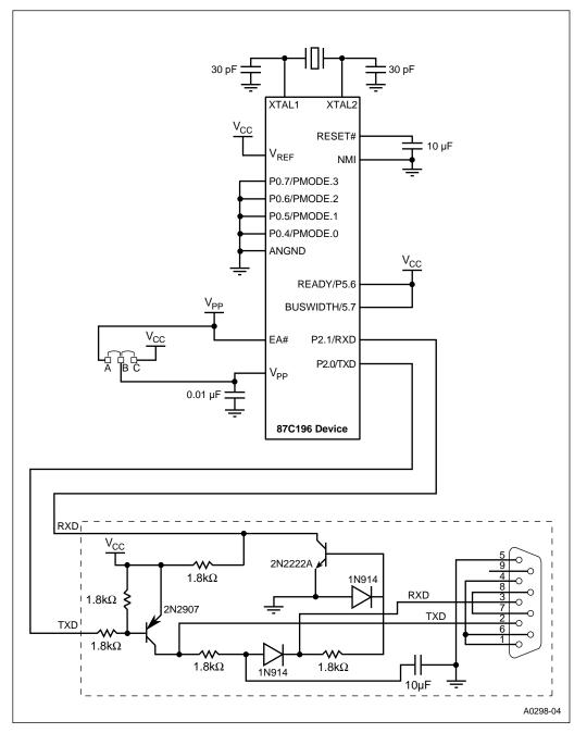
Figure 15-14. Serial Port Programming Mode Circuit
