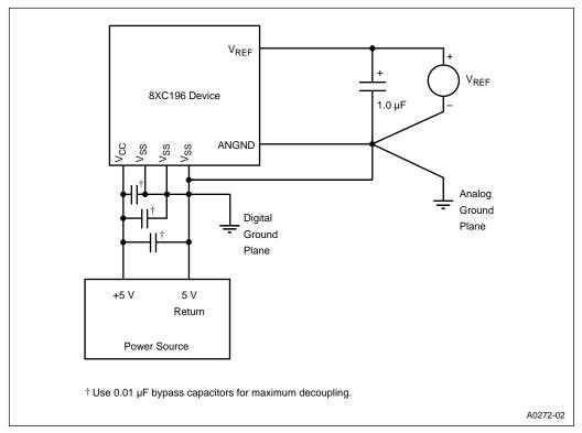
Figure 12-2. Power and Return Connections
