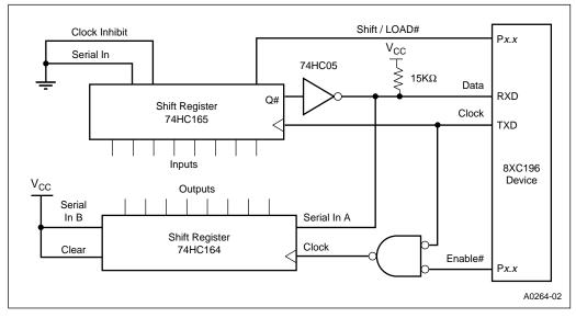
Figure 7-2. Typical Shift Register Circuit for Mode 0
