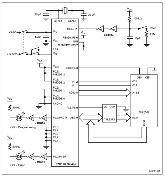
Figure 15-12. Auto Programming Circuit
