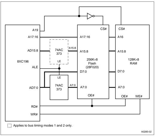
Figure 14-12. 8-bit System with Flash and RAM
