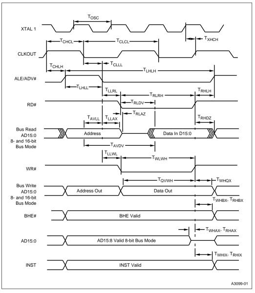
Figure 14-24. Mode 2 System Bus Timing
