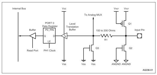
Figure 6-1. Standard Input-only Port Structure
