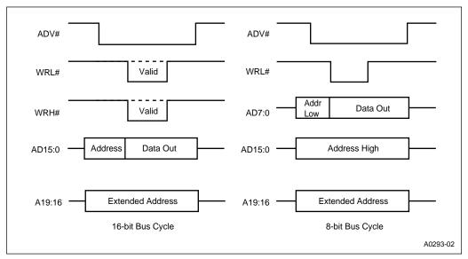
Figure 14-20. Timings of Address Valid with Write Strobe Mode
