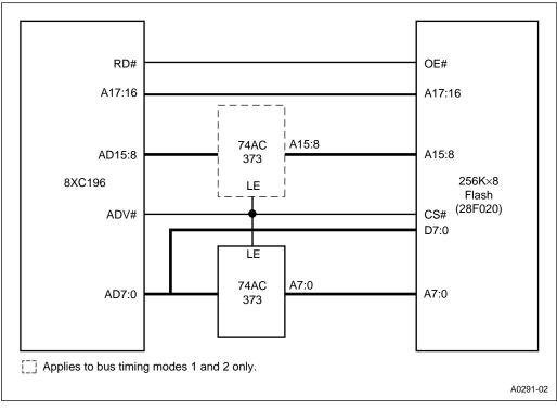
Figure 14-18. 8-bit System with Flash
