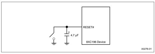
Figure 12-9. Minimum Reset Circuit
