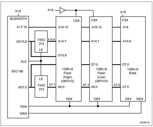
Figure 14-13. 16-bit System with Dynamic Bus Width
