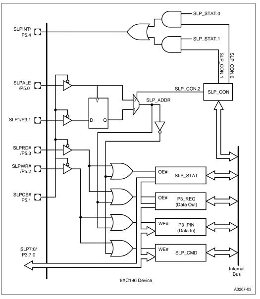
Figure 9-2. Slave Port Block Diagram
