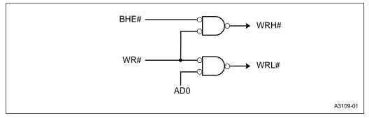
Figure 14-11. Decoding WRL# and WRH#
