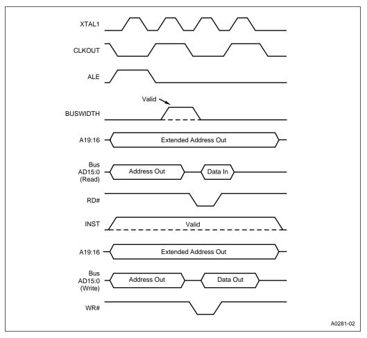
Figure 14-6. Timings for 16-bit Buses
