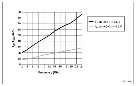
Figure 1. ICC, IIDLE versus Frequency
