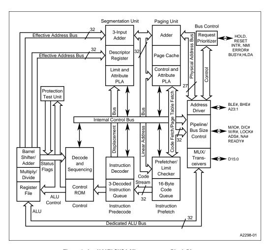
Figure 1. Intel386™ SXSA Microprocessor Block Diagram
