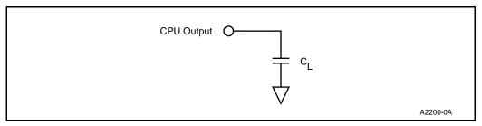
Figure 6. AC Test Loads
