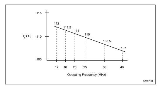
Figure 4. Case Temperature vs. Frequency at  $T_{\rm J}$  = 115° C
