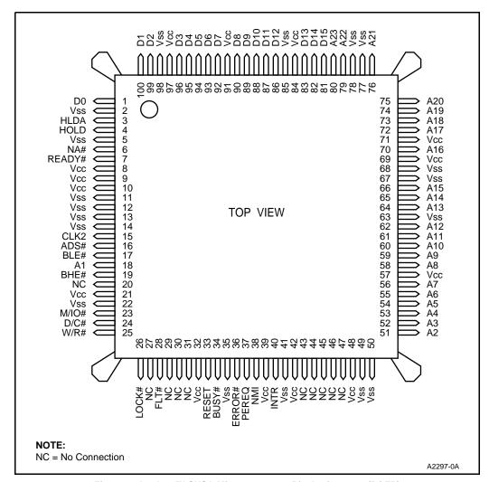
Figure 2. Intel386™ SXSA Microprocessor Pin Assignment (PQFP)
