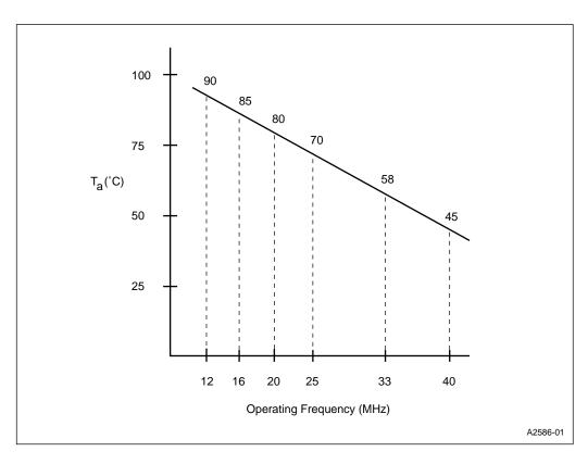
Figure 3. Ambient Temperature vs. Frequency at Zero Air Flow and  $T_{\scriptscriptstyle J}$  = 115° C
