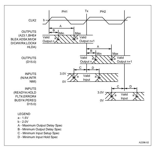
Figure 5. Drive Levels and Measurement Points for AC Specifications
