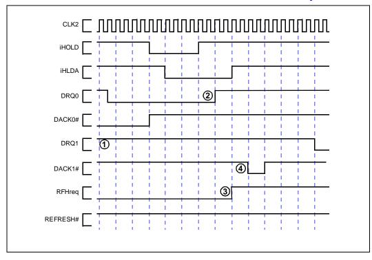
Figure 6. Two DMA Channels in Cascade Mode with Internal RCU Anomaly
