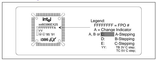
The B-stepping production version of the Special Environment Intel386 EX is designated with a change indicator of '1' or '2'. Figure 2 is an illustration indicating where the change indicator marking is located on the package markings. The change indicator is used to relate information found here, and in other documents like datasheets, to a specific device.
