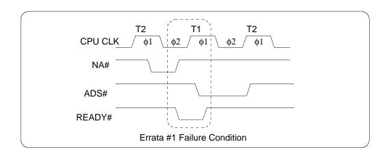
The errata condition is caused by the system generating READY# immediately after NA# has been requested, and a T1 cycle is generated (rather than a T2P cycle). Essentially, the system is requesting a pipelined access, but does not need it because READY# has been returned. Such a condition is not typically expected when using the pipeline feature.
