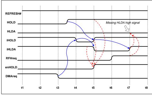
Figure 5. DMA, HOLD and REFRESH with Normal Interval
