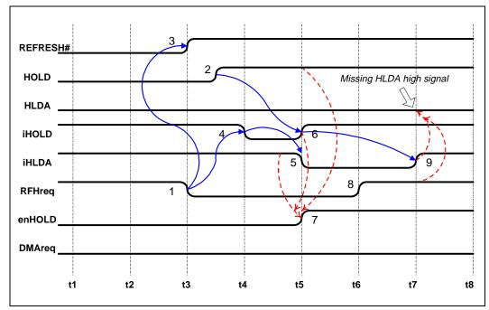
b. HOLD is removed and reasserted within one bus cycle. Refer to Figure 4. This condition will cause the problematic window with fast iHOLD deassertion (t4) and assertion (t5). Note that if HOLD is deasserted because of pending REFRESH and reasserted again within one bus cycle, the problem will not occur since the iHOLD signal is never deasserted due to refresh. The reassertion of the HOLD would then be serviced upon completion of the refresh.
