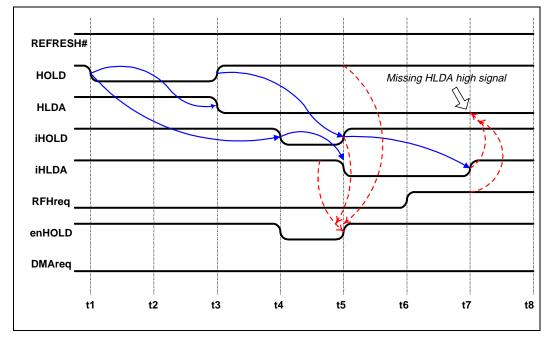
Figure 4. Quick HOLD Assert and Deassert with Slow REFRESH Interval
