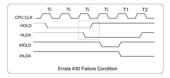
It is also possible for the following to occur when HOLD/HLDA arbitration is an issue: HOLD is driven active during the T1 or Tw of a valid bus cycle. The processor begins the next bus cycle and generates HLDA. HLDA is active for only one T-state. ADS# is extended through the bus cycle. The alternate bus master sees the HLDA and performs its bus activity. HOLD is then driven inactive and the bus is returned to the Intel386<sup>TM</sup> EX Processor. At this point there is bus contention.
