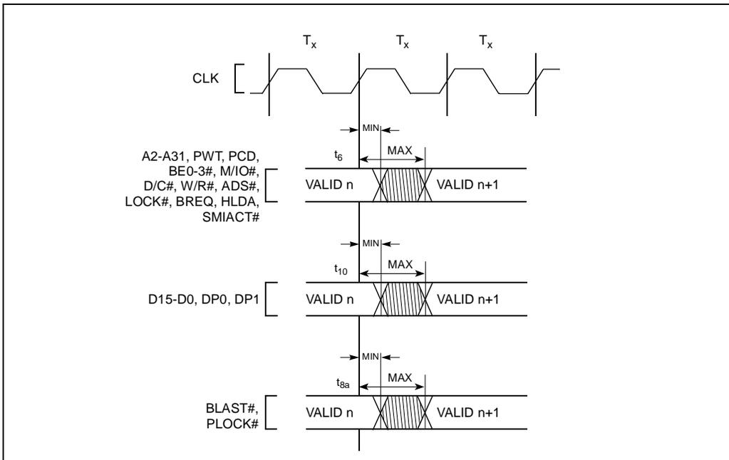
Figure 12. Output Valid Delay Timing
