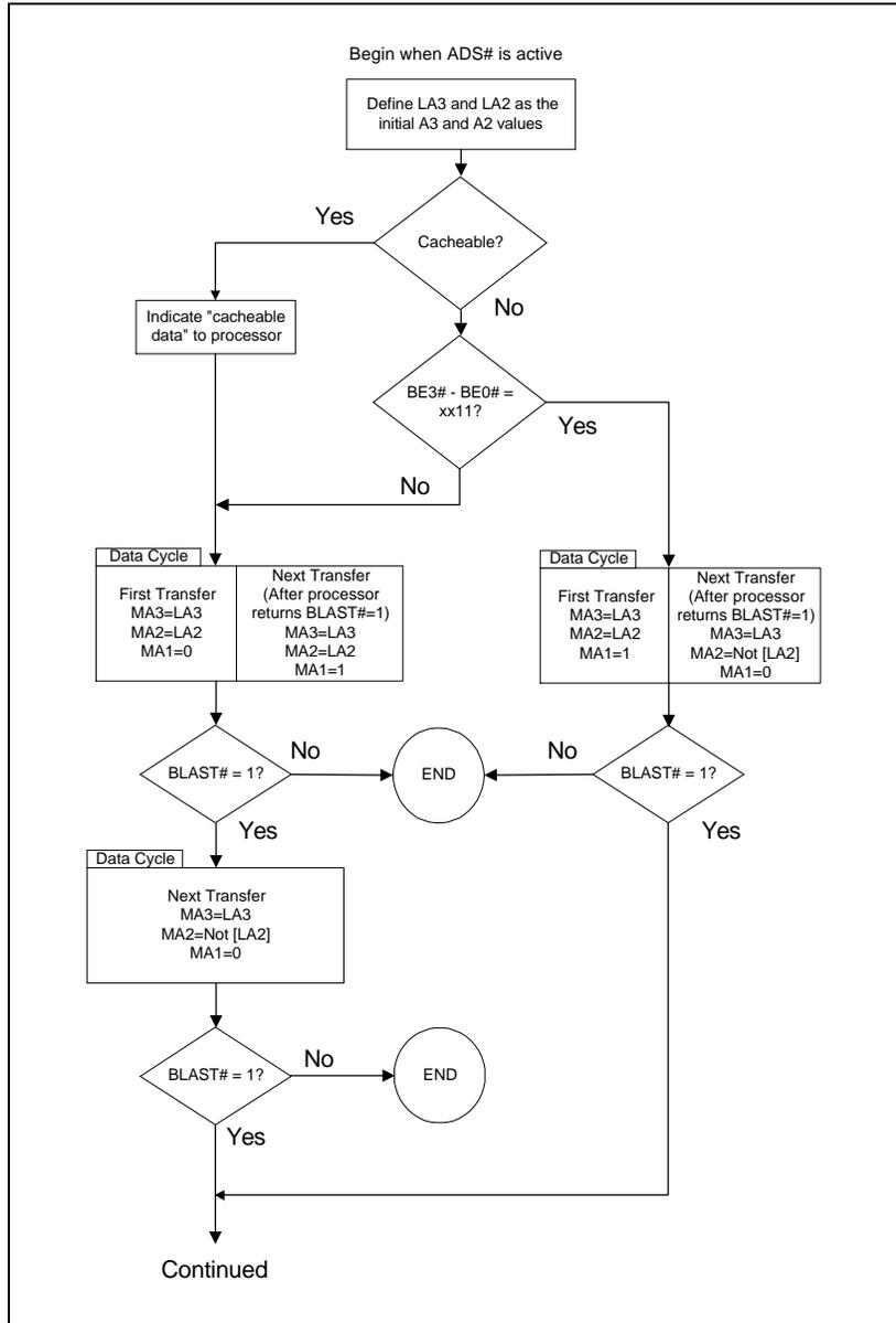
Figure 6. Address Prediction for Burst Transfers (1 of 3)
