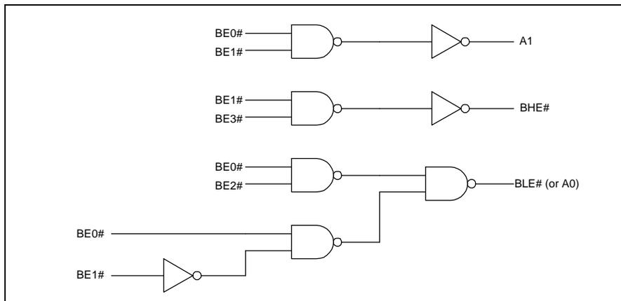
Figure 5. Logic to Generate A1, BHE# and BLE#
