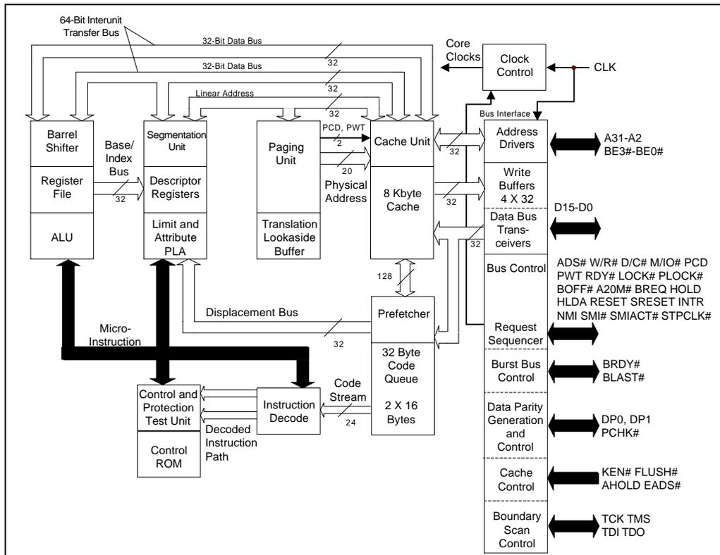
Figure 1. Embedded ULP Intel486™ GX Processor Block Diagram
