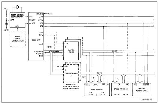
Figure 4a. Minimum Mode 8086 Typical Configuration
