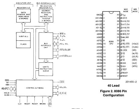
Figure 1. 8086 CPU Block Diagram
