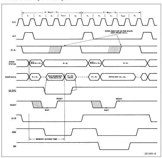
Figure 5. Basic System Timing
