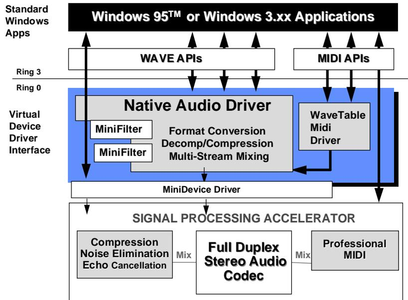
The Native Audio architecture is extensible in both hardware and software. Extensibility in software is provided in three ways:
