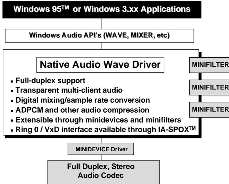
From an architectural point of view, Native Audio represents the application of NSP technology to audio to create a Windows Wave driver. It functions as a virtual device driver within the Windows operating system. Native Audio is a Windows MMSYSTEM device driver that implements the WAVE and MIXER APIs and executes the requested function in software on the processor. In turn, the Native Audio driver then works directly with the audio hardware (codec).
