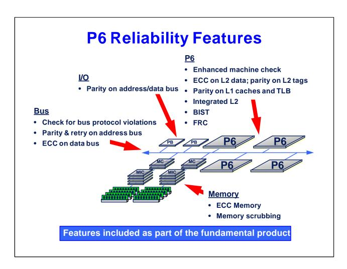
A key design objective of the P6 and its chipset was to include the features required as a foundation for reliable system design.
