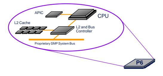
Integrating the CPU, L2 cache, APIC and Bus controller into a single package makes the P6 a unique multiprocessing building block element. The P6 bus is a cache-coherent, transaction oriented bus that scales to four processors even under the worst benchmark loading scenarios (TPCs). Also, the board area taken by the P6 is less than a Pentium® processor plus it's L2 cache.
