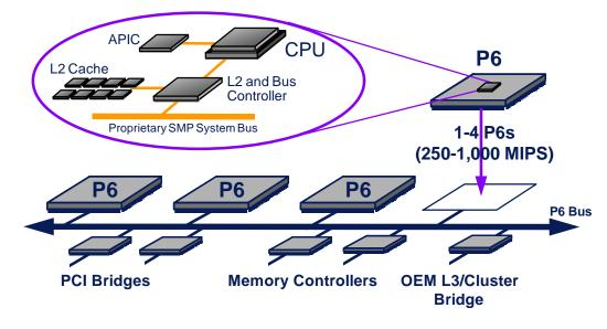
The P6 chipset is designed to allow independent scaling of CPU, memory and I/O.
