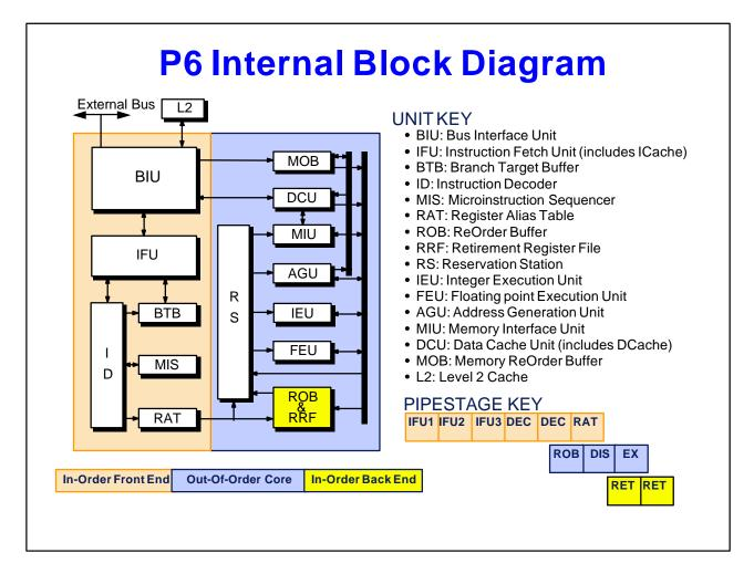
IFU does all the prefetching, and predecode, in pipestages IF1, IF2 and IF3 ID decodes the instructions into micro-operations (uops), in pipestages DEC,DEC RAT allocates destination registers for each uop
