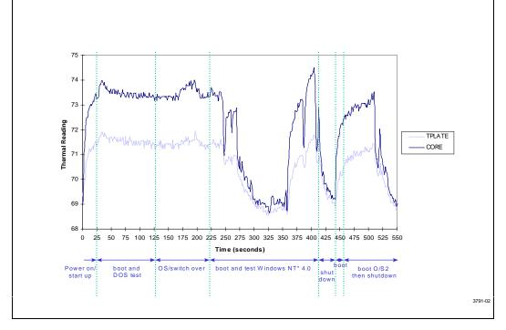
As the above figure illustrates, the  $T_{PLATE}$  response lags  $T_{CORE}$  and the swings in  $T_{CORE}$  are typically larger than the swings in  $T_{PLATE.}$
