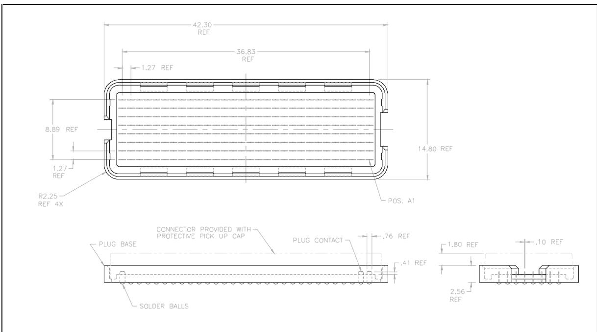
**Figure 1. 240-Position BGA Connector (Plug Assembly)
