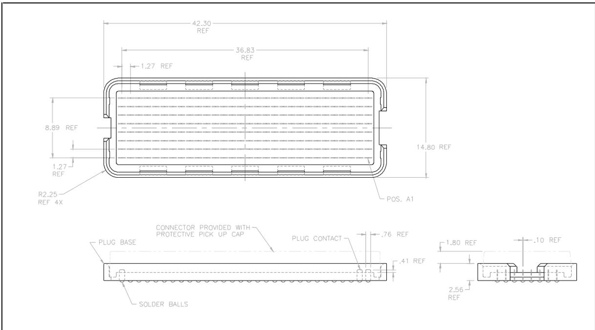
**Figure 1. 240-Position BGA Connector (Plug Assembly)
