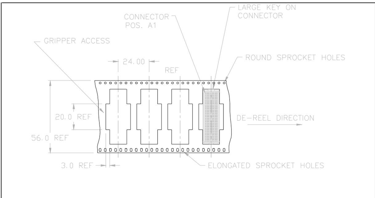
Figure 4. Tape and Reel Packaging (Dimensions in mm)
