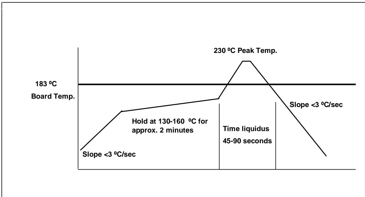
Figure 6. Typical Oven Reflow Profile (not to scale)
