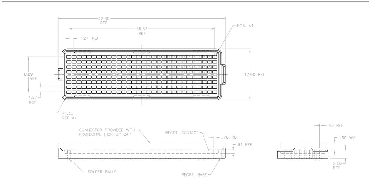
**Figure 2. 240-Position Connector (Receptacle Assembly)
