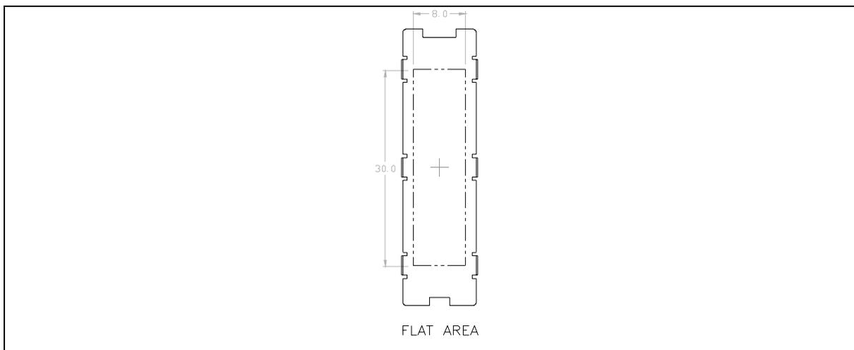
Figure 5. Vacuum Pick-Up Cap (Dimensions in mm)
