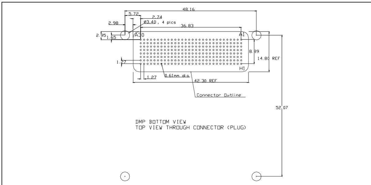
**Figure 3. 240-Position Connector Footprint (Dimensions in mm)**
