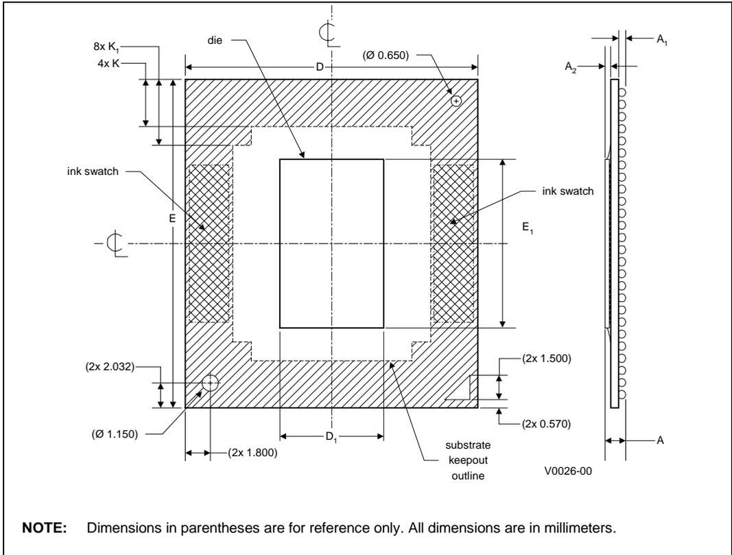
Figure 5.1 Surface-Mount BGA1 Package-Top and Side View
