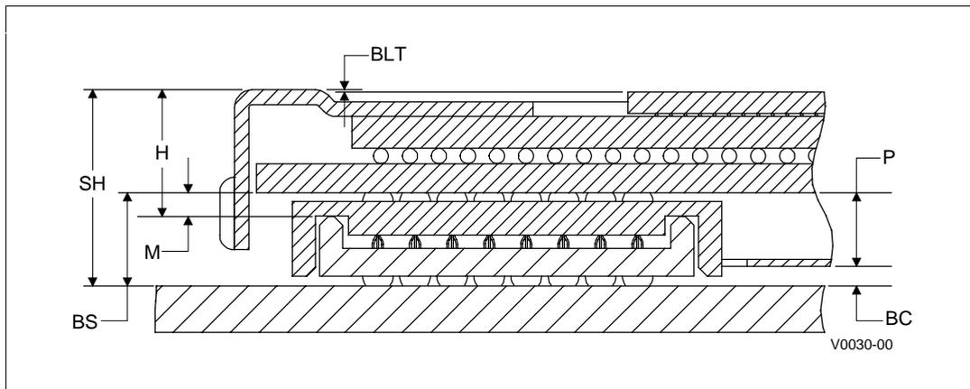
**Figure 5.6 Mini-Cartridge Cross-Section with Vertical Dimensions**
