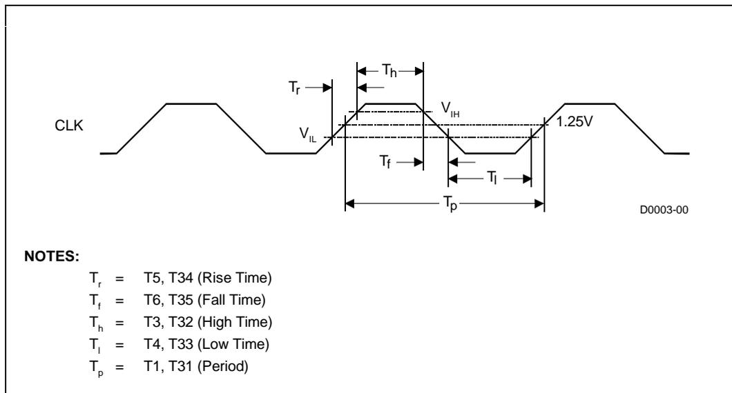
Figure 3.2 Generic Clock Waveform
