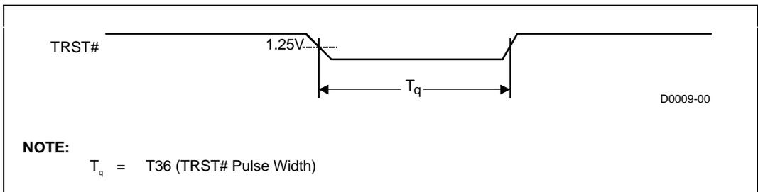
Figure 3.8 Test Reset Timings
