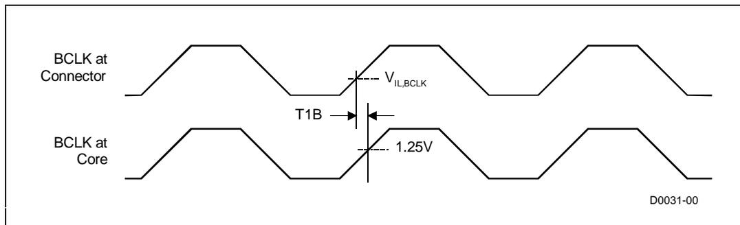
Figure 3.1 BCLK Connector to Core Offset
