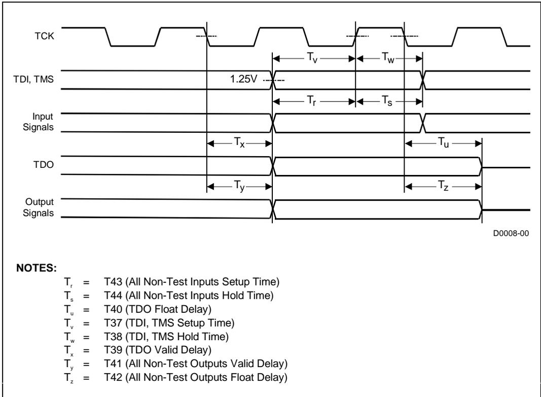
Figure 3.7 Test Timings (Boundary Scan)
