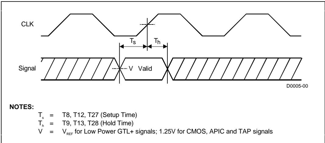
**Figure 3.4 Setup and Hold Timings**
