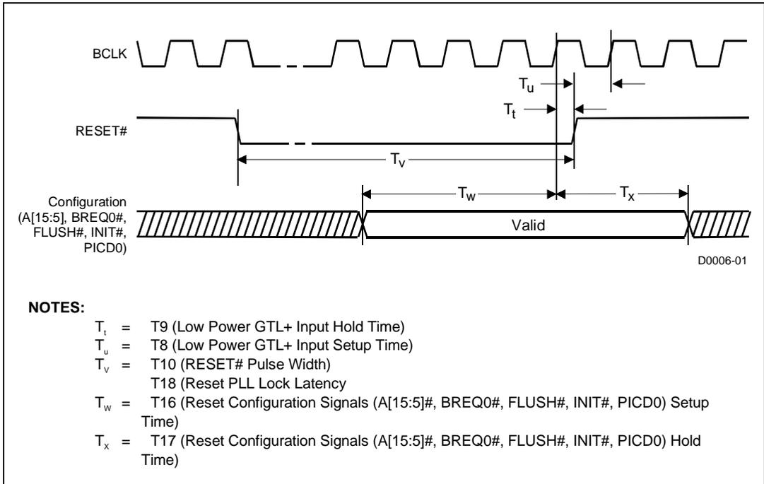
**Figure 3.5 Cold/Warm Reset and Configuration Timings**
