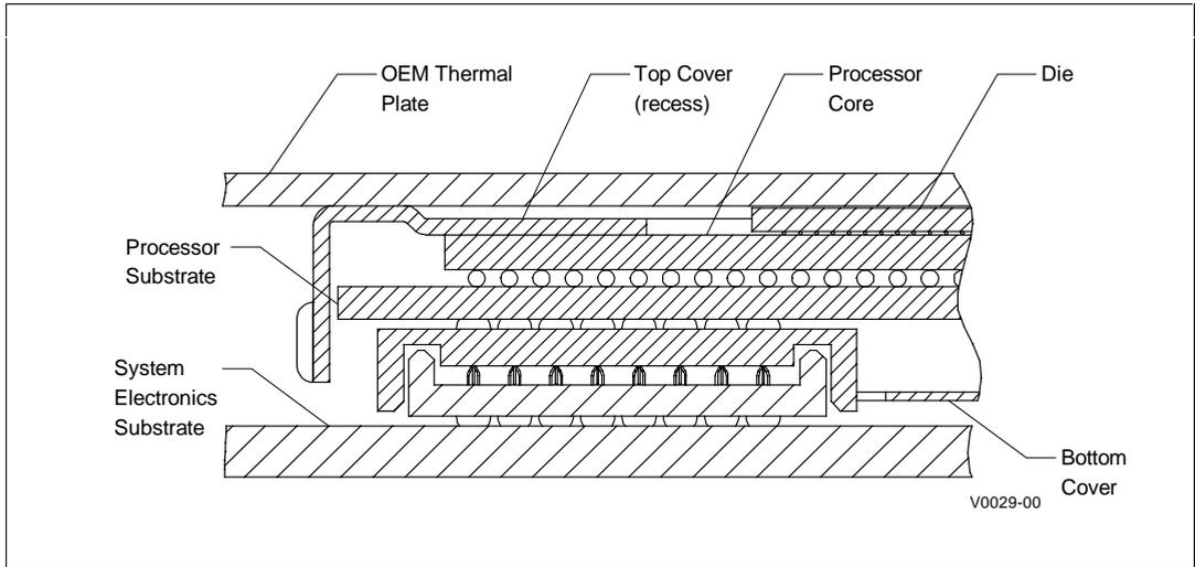
**Figure 5.1 Mini-Cartridge Cross-Section View**
