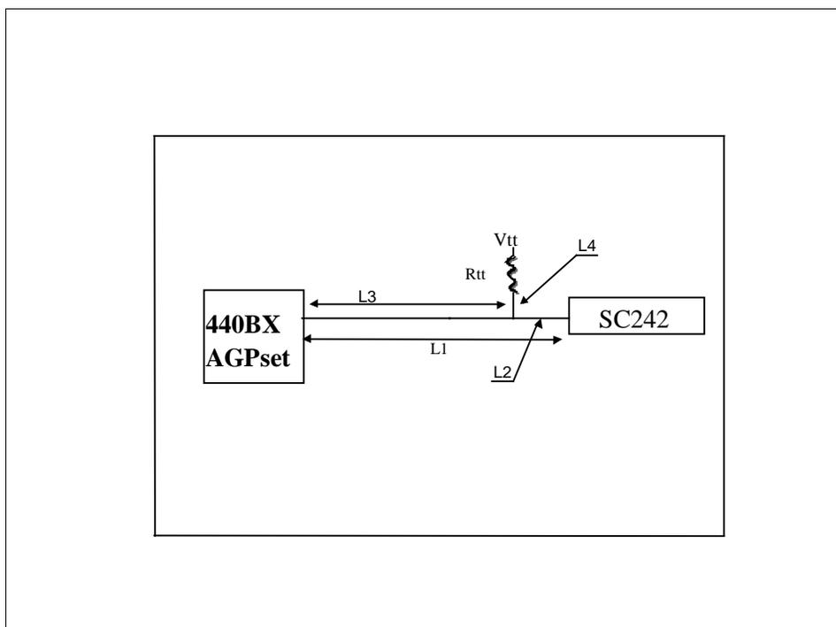
Figure 15. Recommended topology for single processor design
