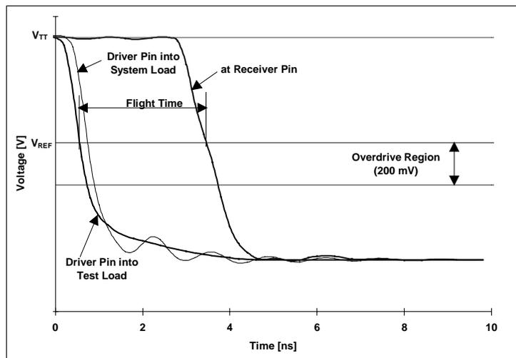
**Figure 13. Example falling edge flight time measurement**
