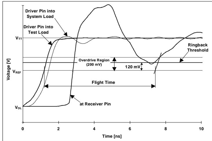
**Figure 12. Flight time measurement with non-monotonic rising edge**
