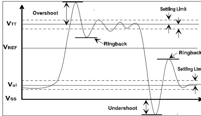
**Figure 14. Overshoot, ringback, and settling time**
