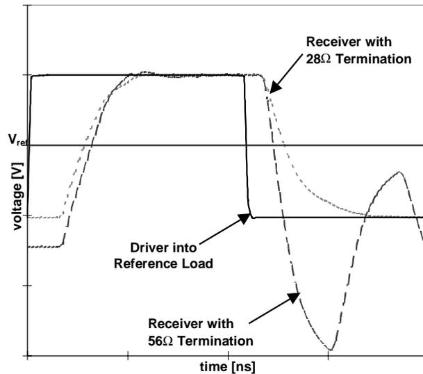
Figure 2. AGTL+ flight time dependence on  $R_{TT}$ .
