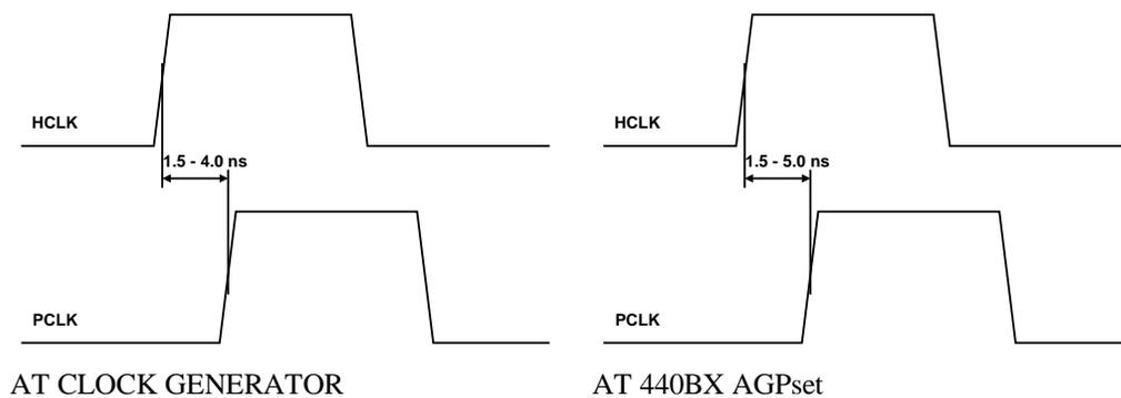
Figure 25. Host-to-PCI clock lag spec
