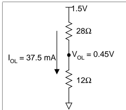
**Figure 4. Equivalent circuit for output low state.**
