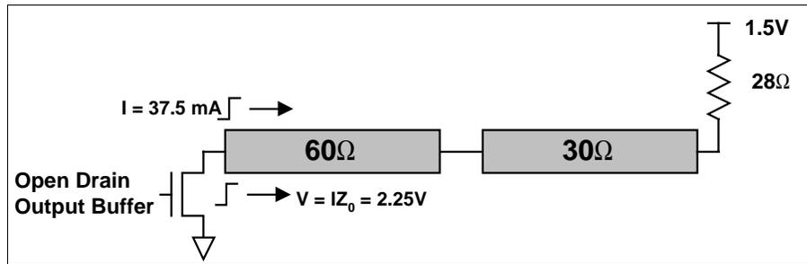
Figure 5. Waveform launch for low-high signal transition.
