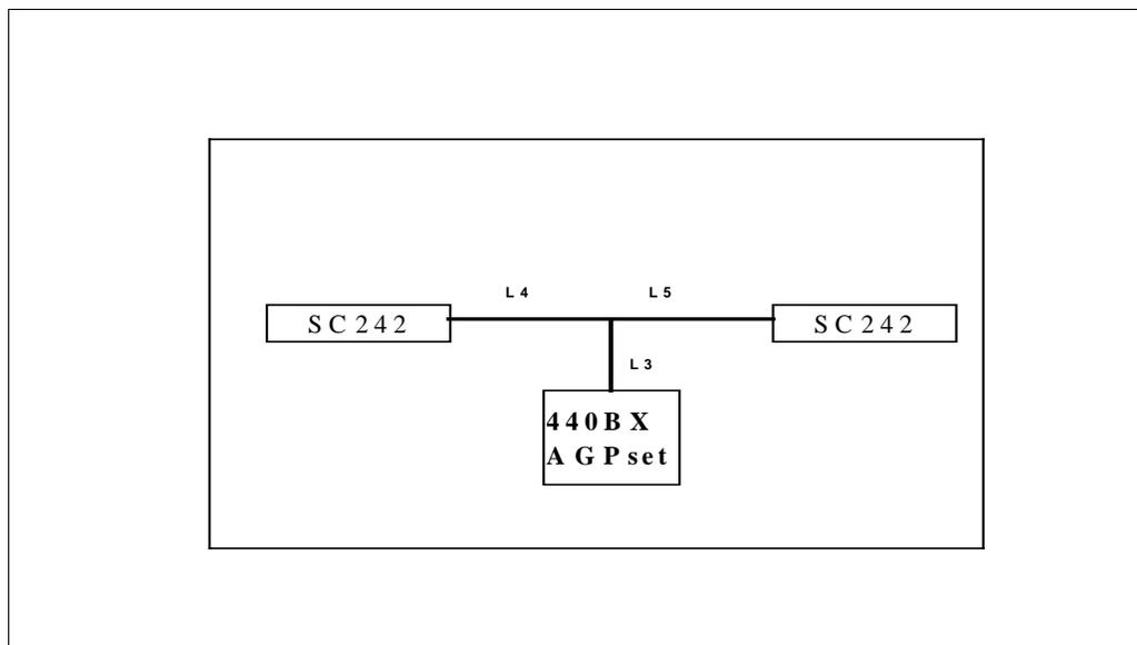
Figure 21. Recommended topology for dual processor design
