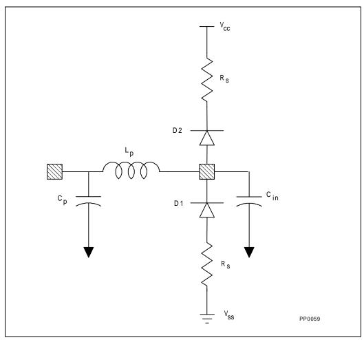
Figure 24-1. Input Buffer Model, Except Special Group
