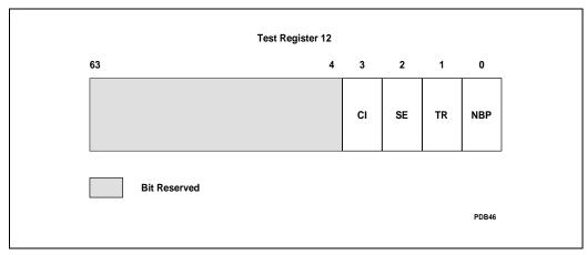
Figure 13-1. Test Register TR12
