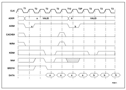
Figure 6-17. Two Pipelined Cache Line Fills
