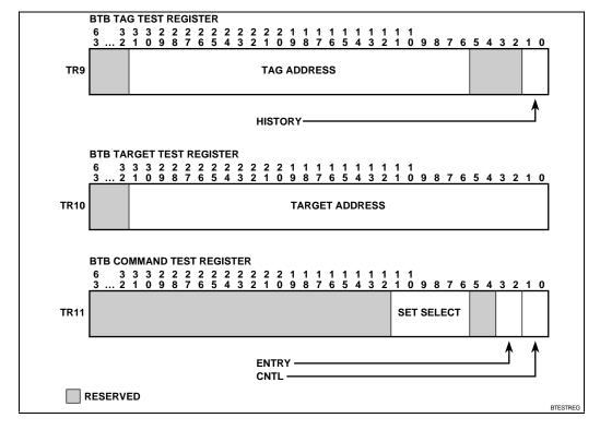
Figure 33-3. BTB Test Registers
