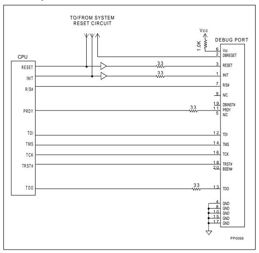
Figure 31-2. Single CPU — Boundary Scan Not Used
