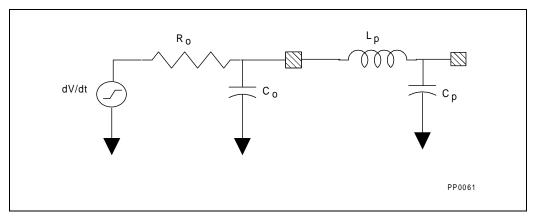
Figure 24-3. First Order Output Buffer Model
