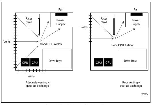
Figure 16-9. Airflow Design Examples
