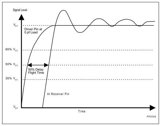
Figure 23-8.  $V_{cc}$  Measurement of Flight Time
