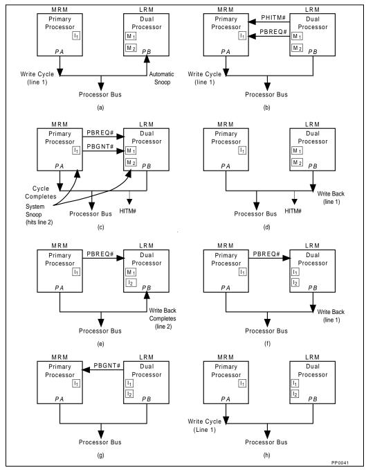
Figure 20-8. DP Cache Consistency for External Snoops
