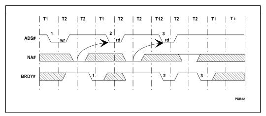
Figure 6-30. Bus Cycles Without Dead Clock
