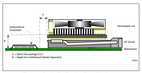
Figure 16-7. Required Free Space from Sides of PGA Package
