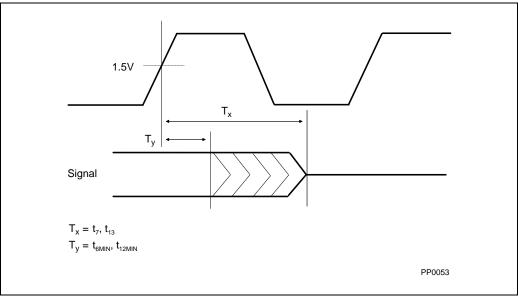
Figure 23-3. Float Delay Timings
