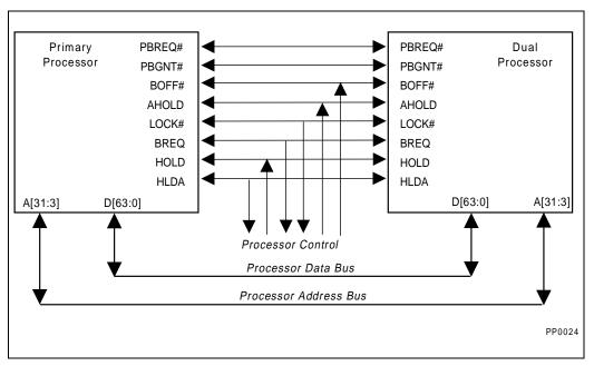
Figure 20-2. Dual Processor Arbitration Interface
