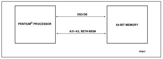
Figure 6-3. Pentium® Processor with 64-Bit Memory
