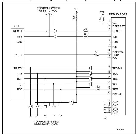
Figure 31-3. Single CPU — Boundary Scan Used
