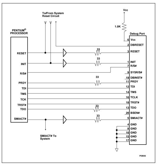
Figure 15-2. Minimal Debug Port Implementation
