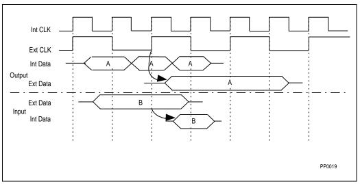
Figure 19-2. Pentium® Processor (610\75, 735\90, 815\100, 1000\120, 1110\133) 1/2 Bus Internal/External Data Movement
