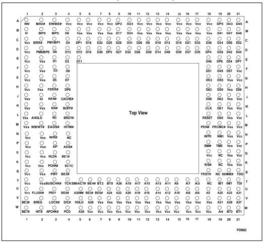
Figure 1-1. Pentium® Processor (510\60, 567\66) Pinout (Top View)
