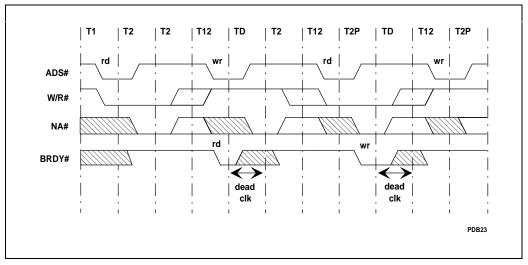
Figure 6-31. Bus Cycles with TD Dead Clock
