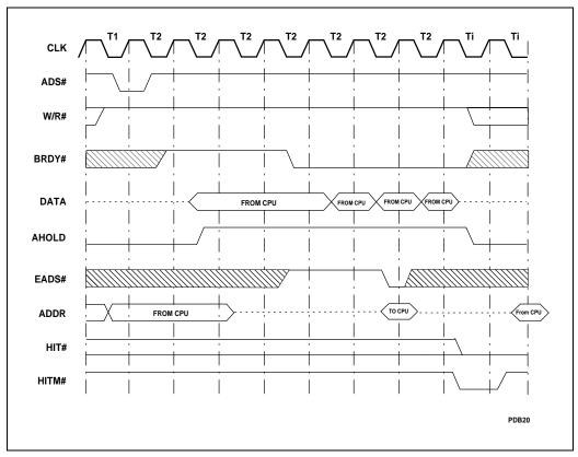
Figure 6-28. Latest Snooping of Writeback Buffer
