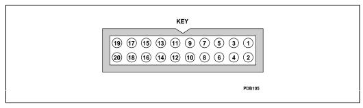
Figure 15-1. Debug Port Connector
