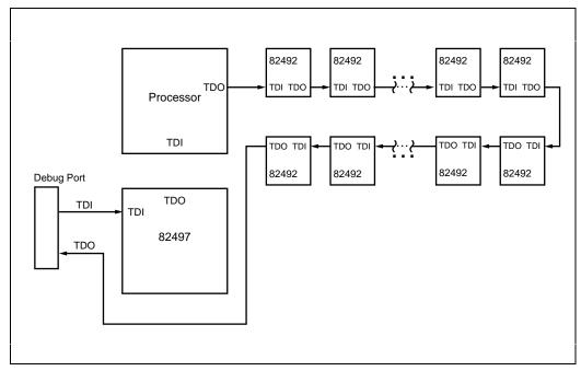
Figure 31-7. Example of Multiple Components in Scan Chain
