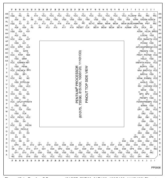
Figure 17-1. Pentium® Processor (610\75, 735\90, 815\100, 1000\120, 1110\133) Pinout — Top Side View
