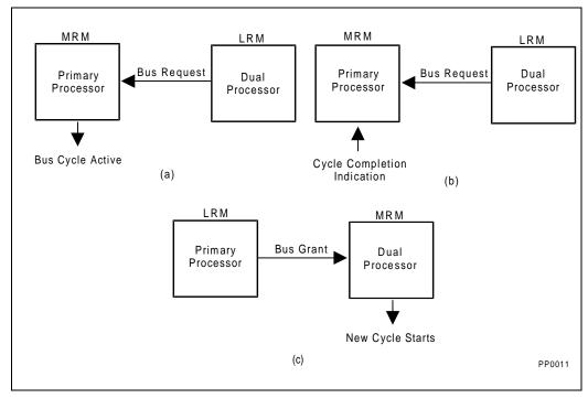
Figure 18-2. Dual Processor Arbitration Mechanism
