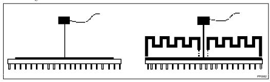
Figure 26-1. Technique for Measuring T<sub>C\*</sub>
