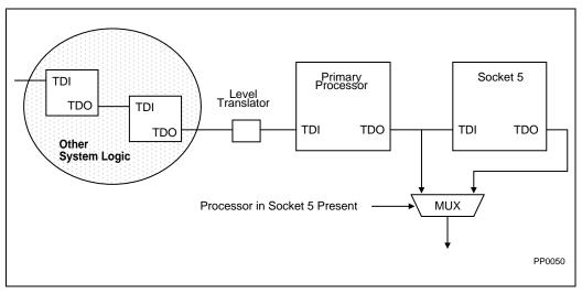
Figure 20-10. Dual Processor Boundary Scan Connections
