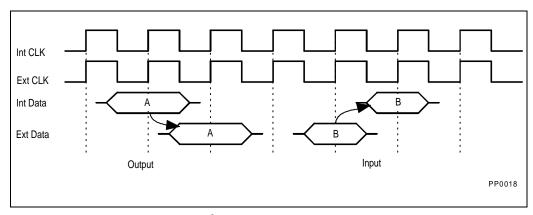
Figure 19-1. Pentium® Processor (510\60, 567\66) Synchronous Internal/External Data Movement
