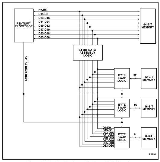
Figure 6-5. Data Bus Interface to 32-, 16- and 8-Bit Memories
