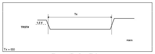
Figure 7-7. Test Reset Timings
