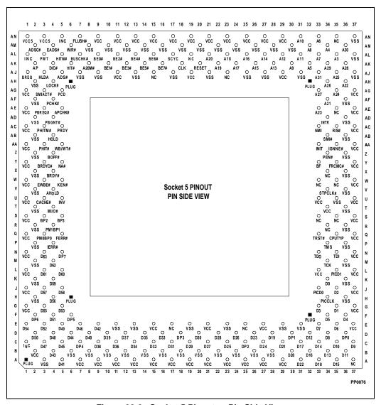
Figure 32-2. Socket 5 Pinout — Pin Side View
