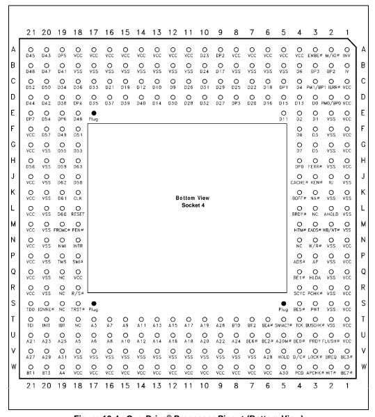
Figure 16-4. OverDrive® Processor Pinout (Bottom View)
