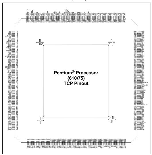
Figure 34-1. Pentium® Processor (610\75) TCP Pinout
