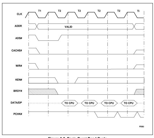
Figure 6-8. Basic Burst Read Cycle
