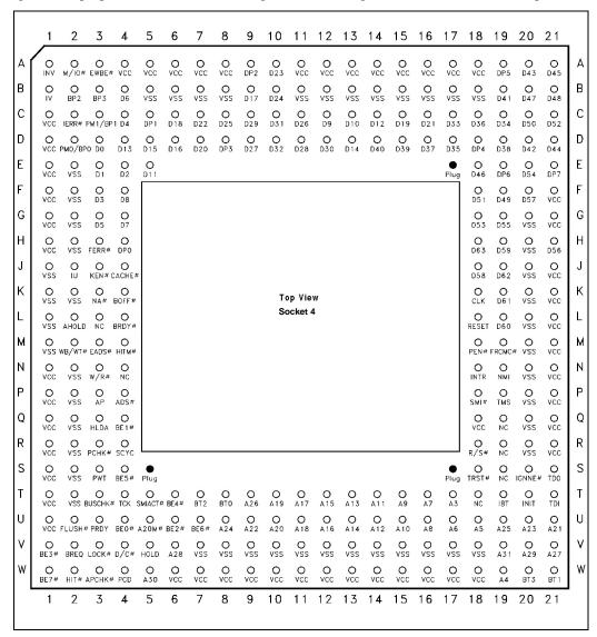
Figure 16-3. Socket 4 Pinout (Top View)
