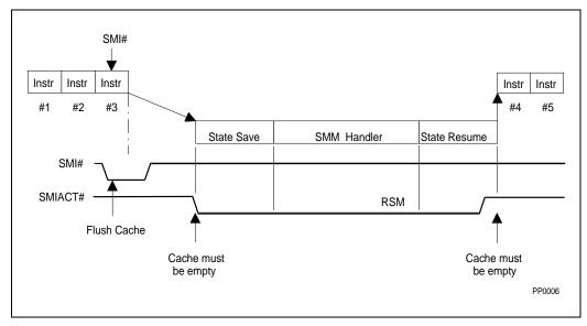
Figure 14-6. FLUSH# Mechanism during SMM with Overlay
