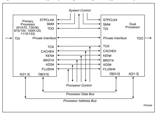
Figure 20-9. Dual Processor Configuration
