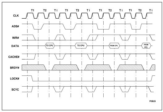
Figure 6-13. Misaligned Locked Cycles
