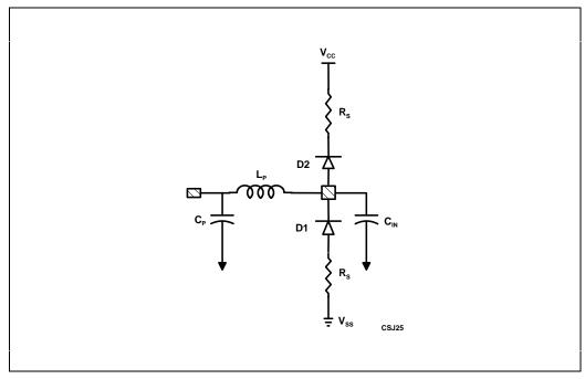
Figure 8-4. Complete Input Model Including Diode
