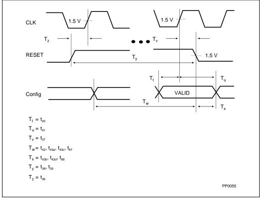
Figure 23-5. Reset and Configuration Timings
