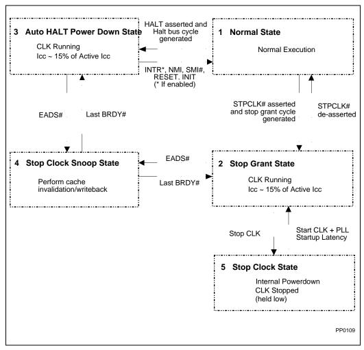
Figure 30-3. Stop Clock State Machine
