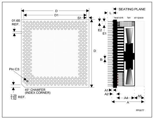
Figure 32-3. Future OverDrive® Processor Package Dimensions
