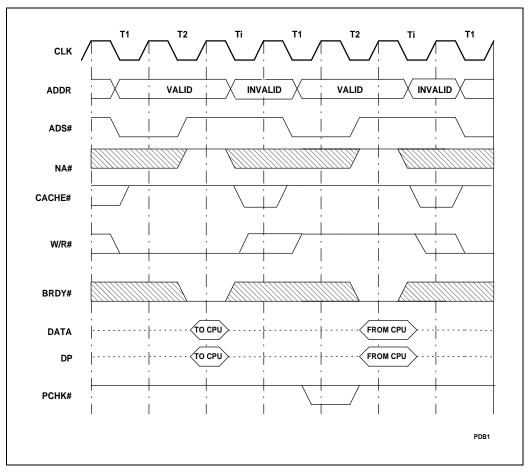
Figure 6-6. Non-Pipelined Read and Write
