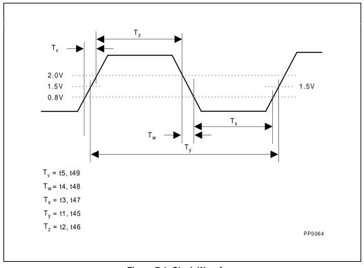
Figure 7-1. Clock Waveform
