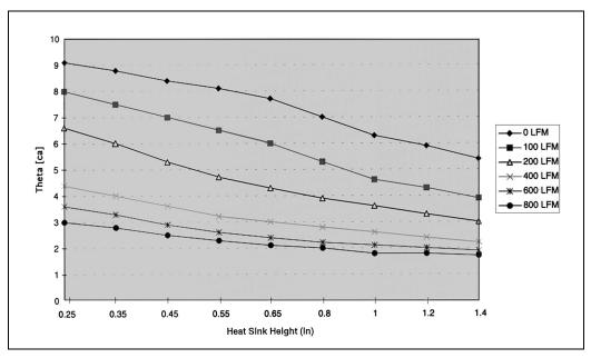
Figure 26-3. Thermal Resistance vs. Heatsink Height (Non-Spreader Package)
