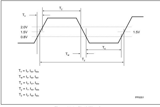
Figure 23-1. Clock Waveform
