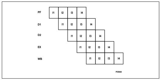
Figure 3-1. Intel486™ CPU Pipe-line Execution
