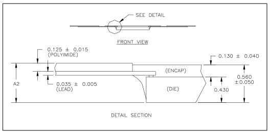
Figure 34-5. One TCP Site (Cross-Sectional Detail)
