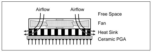
Figure 16-8. Fan/Heatsink Example
