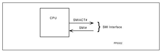
Figure 14-2. Basic SMI# Hardware Interface
