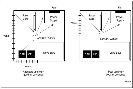
Figure 32-5. Examples of Air Exchange Through PC Chassis
