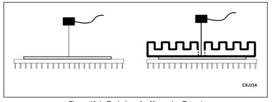
Figure 10-1. Technique for Measuring Tcase\*
