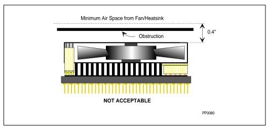
Figure 32-6. Fan/Heatsink Unacceptable Airflow Blockage
