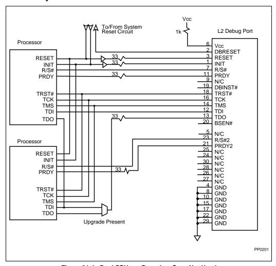
Figure 31-4. Dual CPUs — Boundary Scan Not Used
