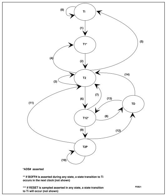
Figure 6-29. Pentium® Processor Bus Control State Machine
