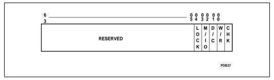
Figure 12-3. Machine Check Type Register
