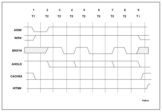
Figure 6-24. AHOLD Restriction during Write Cycles
