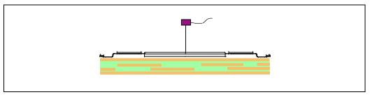
Figure 34-7. Technique for Measuring Case Temperature (T<sub>C</sub>)
