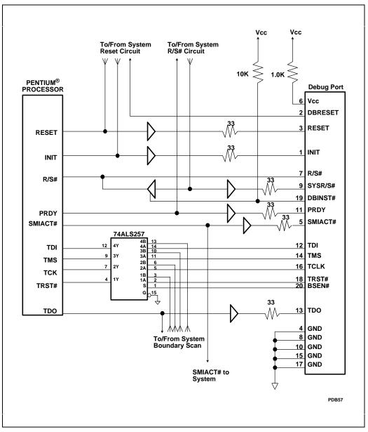
Figure 15-3. Maximal Debug Port Implementation
