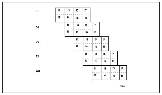
Figure 3-2. Pentium® Processor Pipe-line Execution
