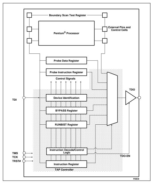
Figure 11-1. Test Access Port Block Diagram
