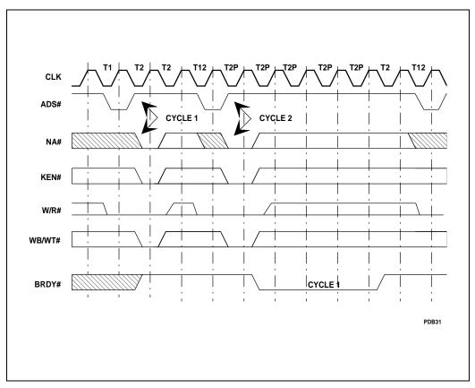
Figure 6-19. KEN# and WB/WT# Sampling with NA#
