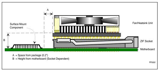
Figure 32-7. Required Free Space from Sides of Chip Package
