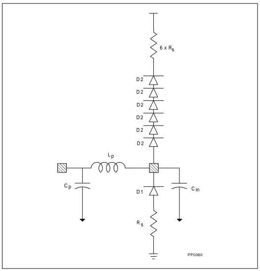
Figure 24-2. Input Buffer Model for Special Group
