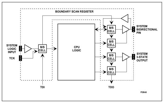
Figure 11-2. Boundary Scan Register
