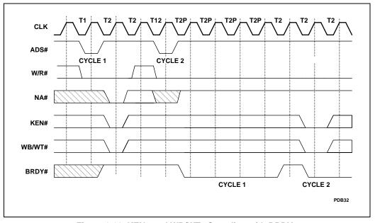
Figure 6-20. KEN# and WB/WT# Sampling with BRDY#
