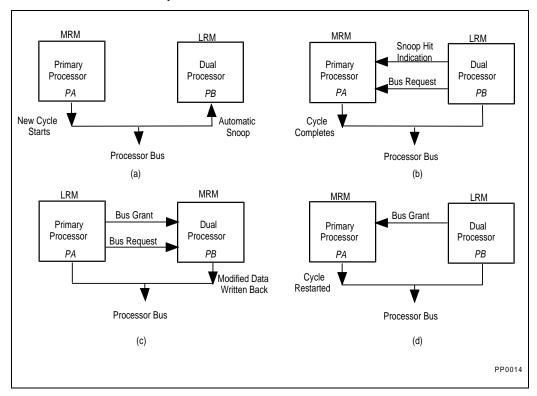
Figure 18-3. Dual Processor L1 Cache Consistency
