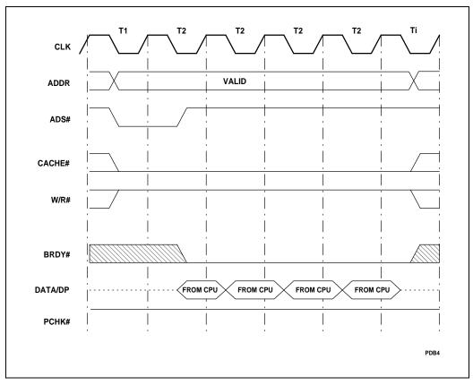
Figure 6-10. Basic Burst Write Cycle
