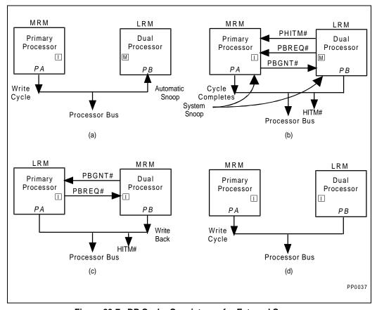
Figure 20-7. DP Cache Consistency for External Snoops
