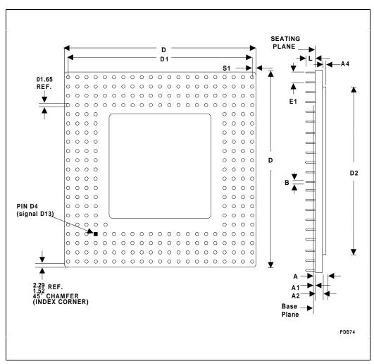
Figure 9-1. Pentium® Processor (510\60, 567\66) Package Dimensions
