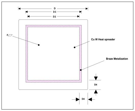
Figure 9-2. Pentium® Processor (510\60, 567\66) Package Dimensions (Top View)
