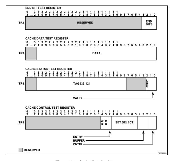
Figure 33-1. Cache Test Registers
