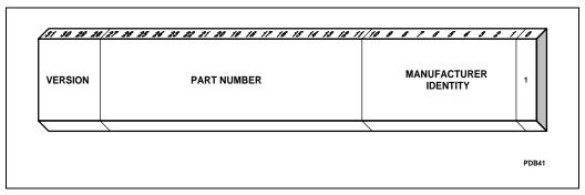
Figure 11-3. Format of the Device ID Register
