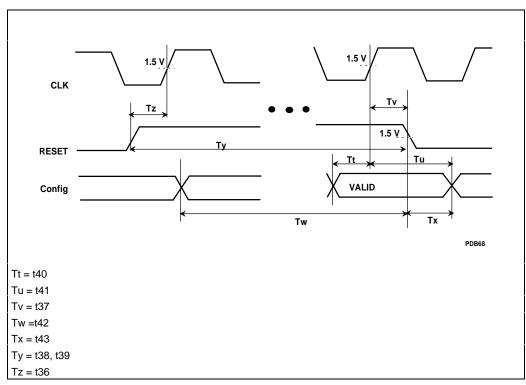
Figure 7-5. Reset and Configuration Timings
