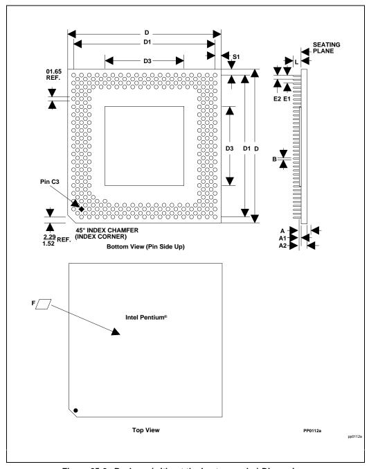
Figure 25-2. Package (without the heat spreader) Dimensions
