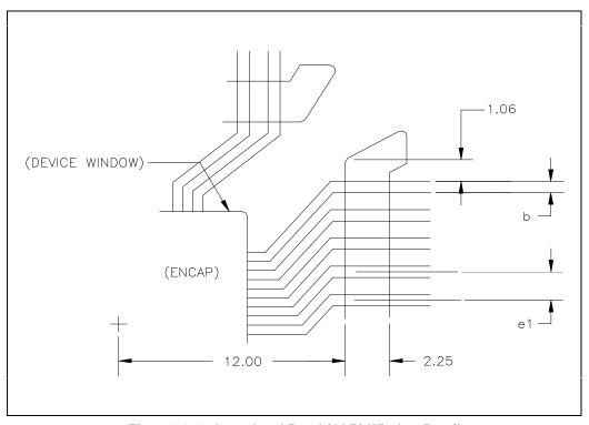
Figure 34-6. Outer Lead Bond (OLB) Window Detail
