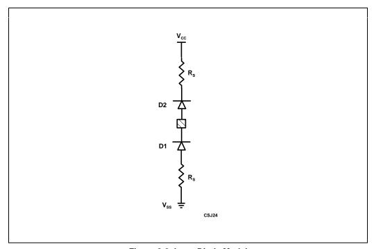
Figure 8-3. Input Diode Model
