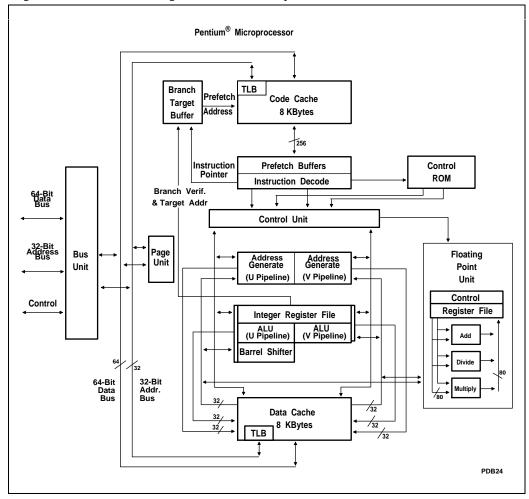
Figure 2-1. Pentium® Processor Block Diagram
