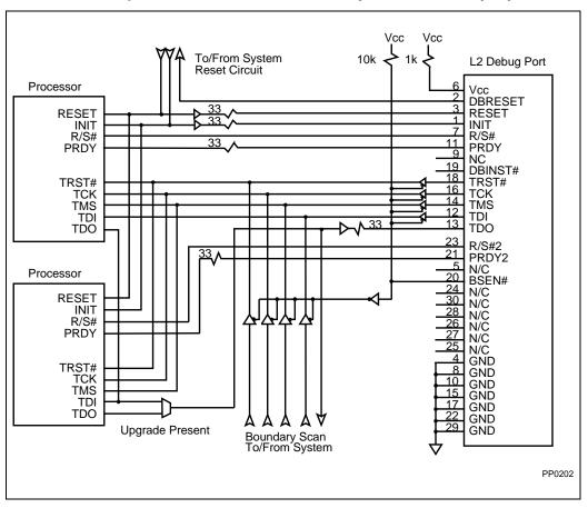
Figure 31-5. Dual CPUs — Boundary Scan Used
