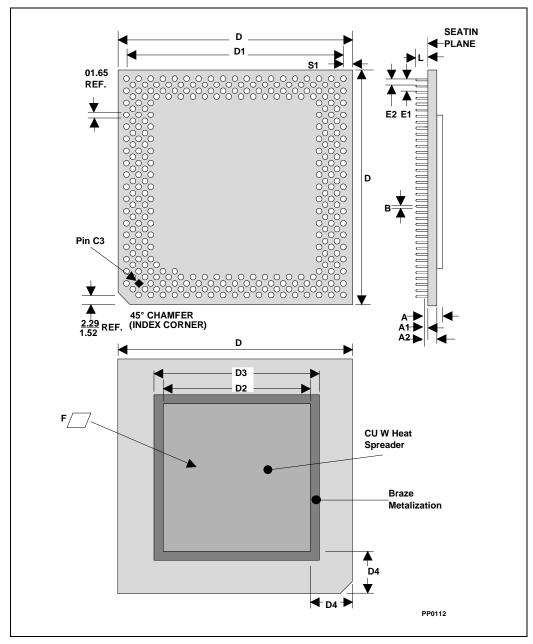
Figure 25-1. Package (with the heat spreader) Dimensions
