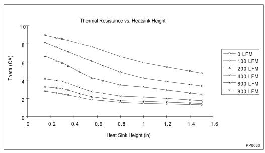
Figure 26-2. Thermal Resistance vs. Heat Sink Height
