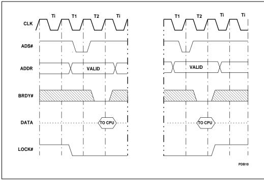
Figure 6-16. Interrupt Acknowledge Cycles
