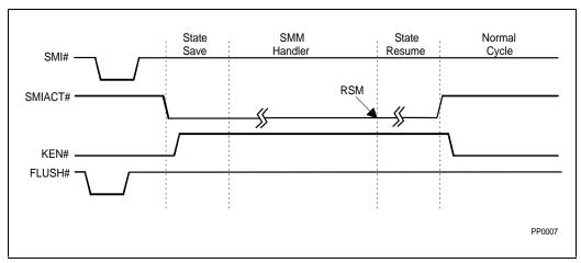
Figure 14-7. Flush with Non-Cached SMM with Overlay
