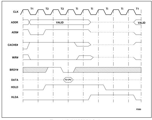
Figure 6-15. HOLD/HLDA Cycles
