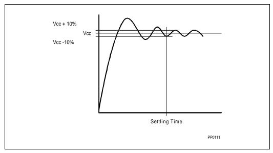
Figure 24-5. Settling Time
