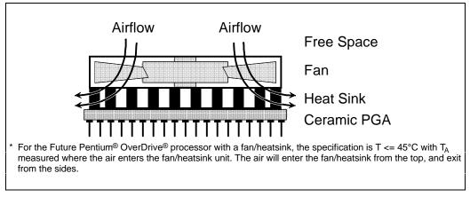
Figure 32-4. Thermal and Physical Space Requirements
