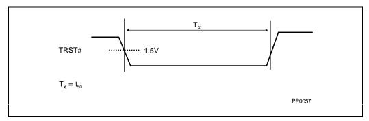
Figure 23-7. Test Reset Timings
