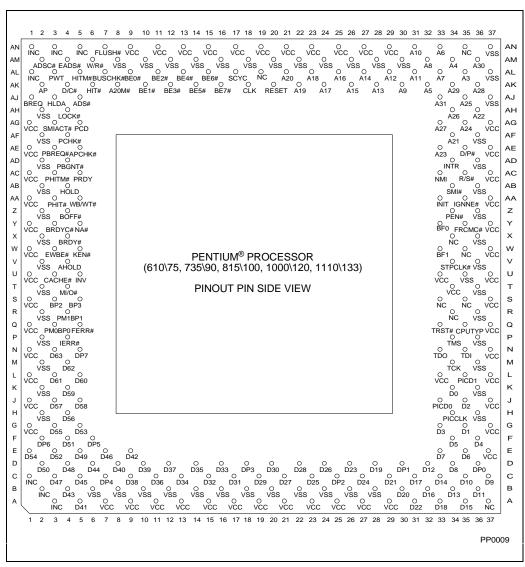
Figure 17-2. Pentium® Processor (610\75, 735\90, 815\100, 1000\120, 1110\133) Pinout — Pin Side View
