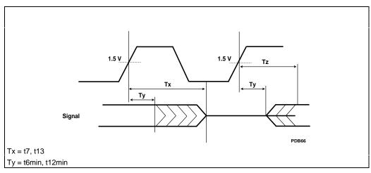
Figure 7-3. Float Delay Timings
