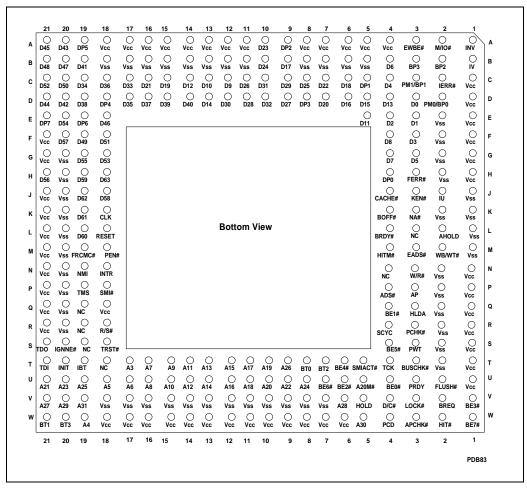
Figure 1-2. Pentium® Processor (510\60, 567\66) Pinout (Bottom View)
