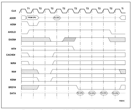
Figure 6-27. Snoop Responsibility Pickup — Pipelined Cycle
