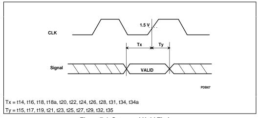
Figure 7-4. Setup and Hold Timings
