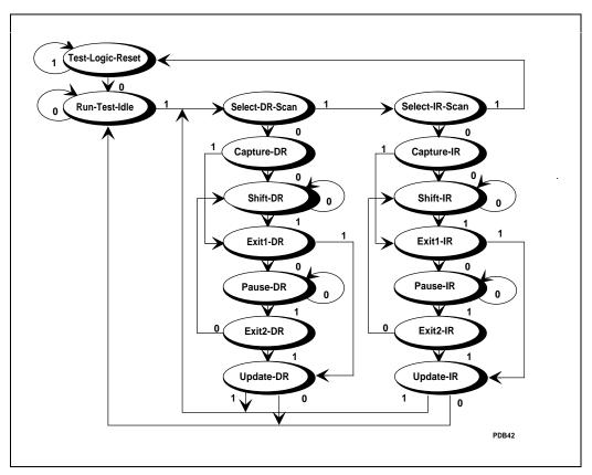
Figure 11-4. TAP Controller State Diagram
