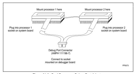
Figure 31-9. Dual Processor Debug Port Adapter
