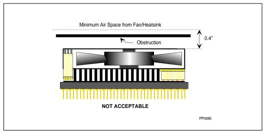
Figure 16-6. Fan/Heatsink Top Space Requirements
