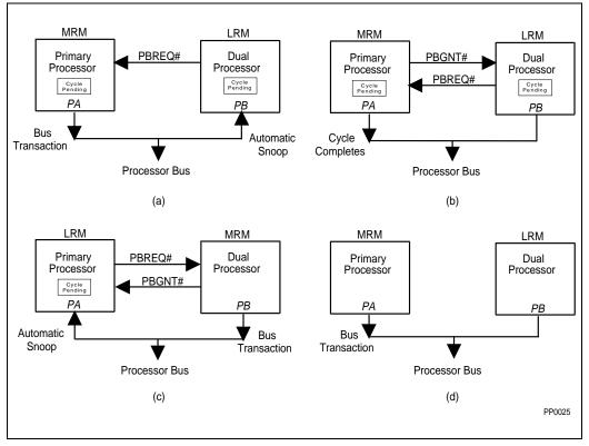
Figure 20-3. Typical Dual Processor Arbitration Example
