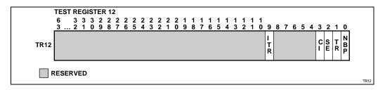
Figure 33-4. Test Register TR12
