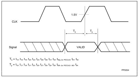
Figure 23-4. Setup and Hold Timings
