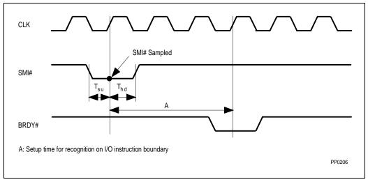
Figure 30-1. SMI# Timing for Servicing an I/O Trap
