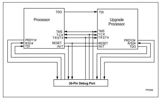
Figure 31-10. Shared Pins for Dual Processor Adapter
