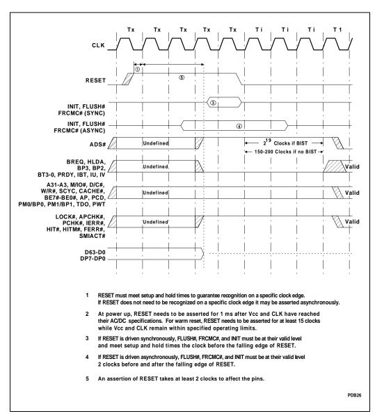
Figure 4-1. Pin States during RESET
