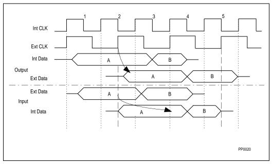
Figure 19-3. Pentium® Processor (610\75, 735\90, 815\100, 1000\120, 1110\133) 2/3 Bus Internal/External Data Movement
