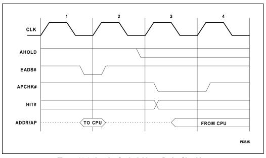
Figure 12-1. Inquire Cycle Address Parity Checking
