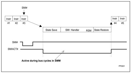
Figure 14-1. Basic SMI# Interrupt Service
