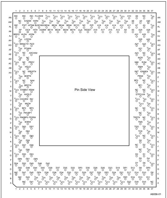
Figure 3. SPGA Pentium<sup>®</sup> Processor with Voltage Reduction Technology Pinout (Pin Side View)
