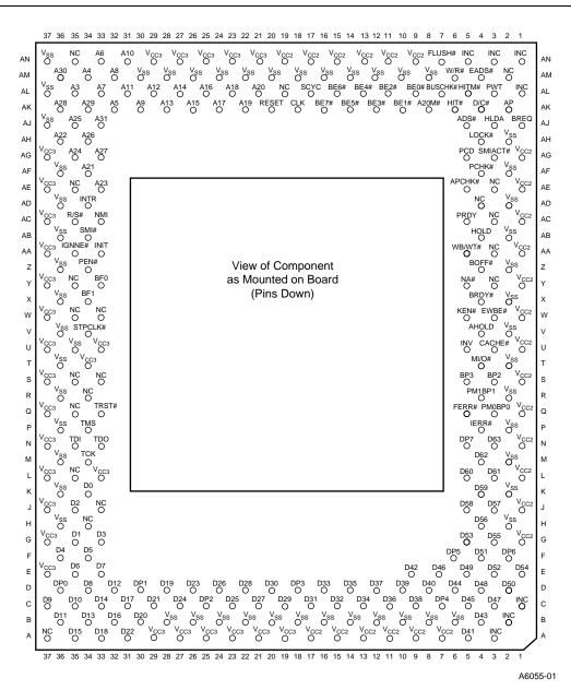
Figure 2. SPGA Pentium<sup>®</sup> Processor with Voltage Reduction Technology Pinout (Top Side View)
