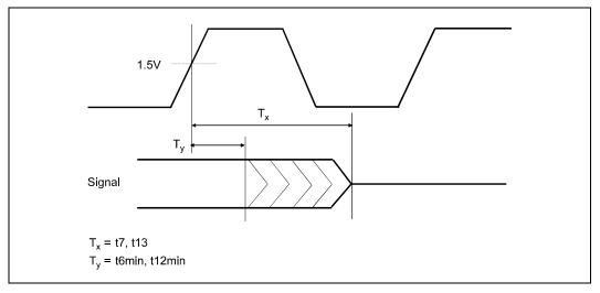
Figure 9. Setup and Hold Timings
