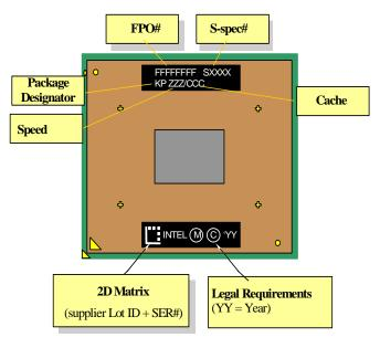
Mobile Intel® Pentium® III Processor-M (Micro-FCPGA) Markings
