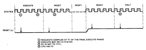
Figure 19: Reset Timing
