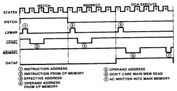
Figure 15: "DCA Indirect" In Control Panel Routine
