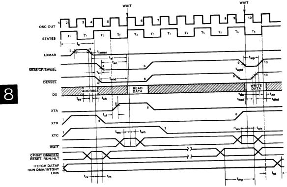
Figure 2: IM6100 AC Timing Diagram
