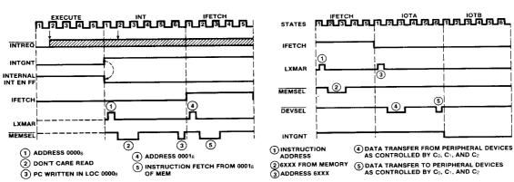
Figure 11: Device Interrupt Grant Timing
