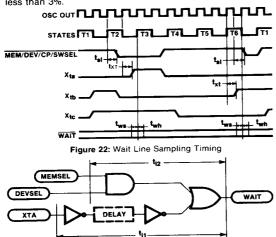
Figure 23: Memory And Input Transfer Wait Circuit
