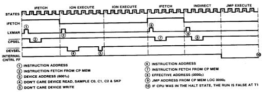
Figure 16: "ION; JMP I 00008" In Control Panel Routine
