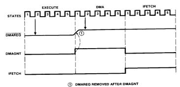
Figure 17: Direct Memory Access (DMA)
