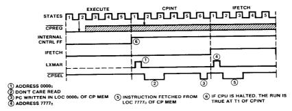
Figure 14: Control Panel Interrupt Grant Timing
