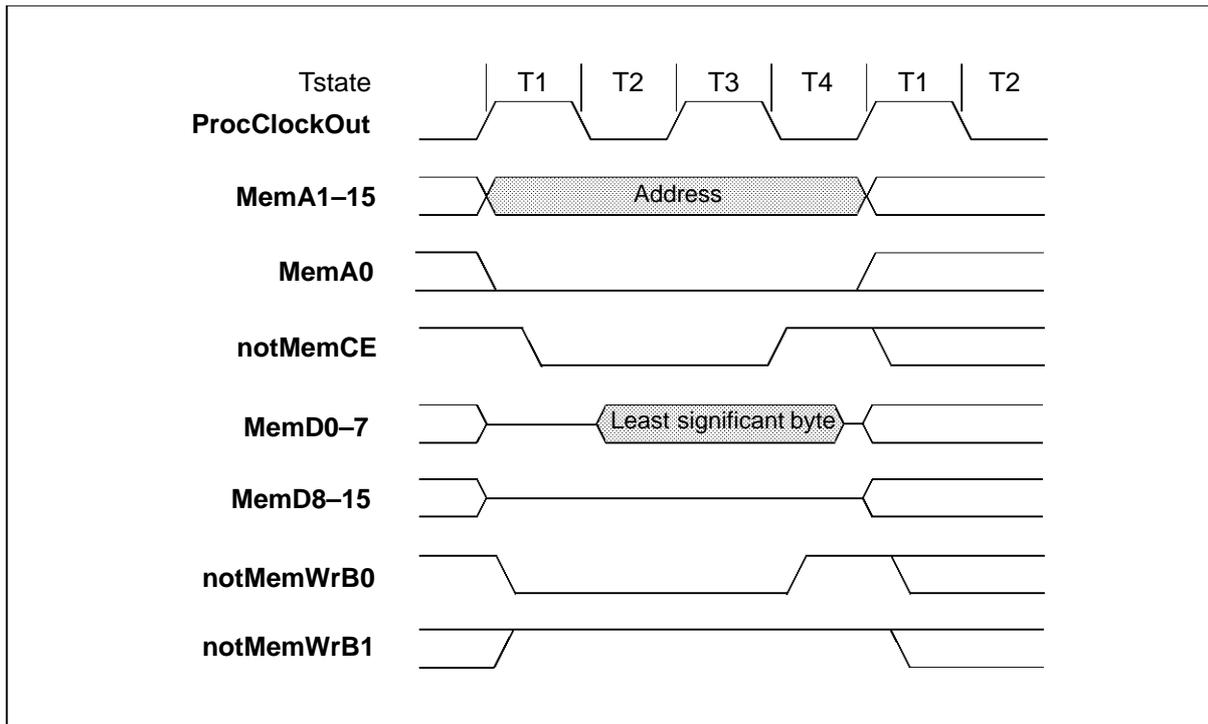
Figure 5.6 IMS T225E least significant byte write in word access mode
