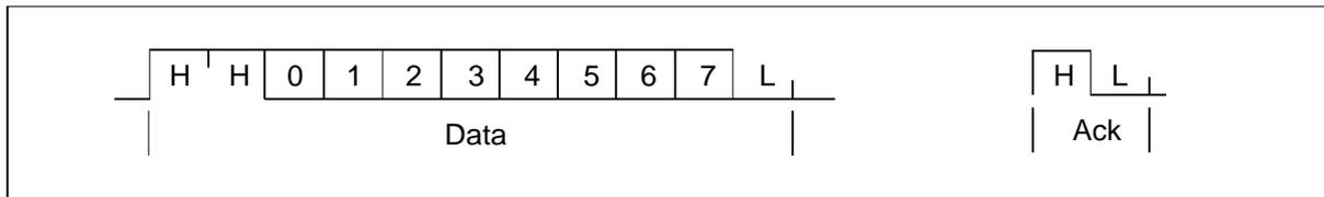
Figure 7.1 IMS T225E link data and acknowledge packets
