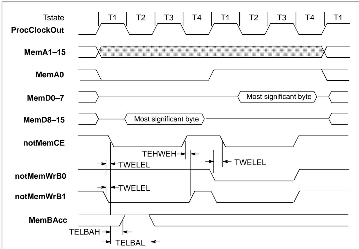
Figure 5.8 IMS T225E most significant byte write to byte-wide memory
