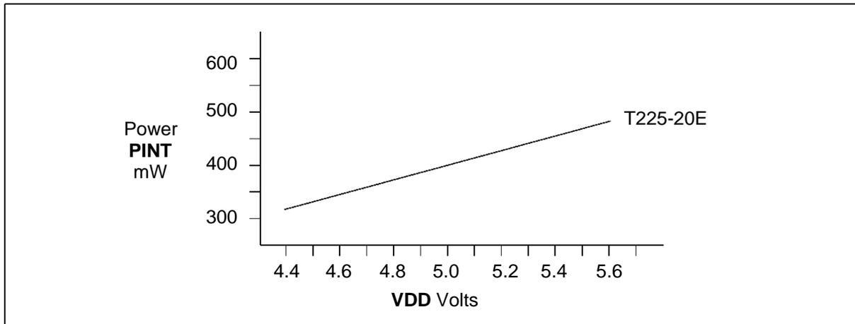
Figure 8.5 IMS T225E internal power dissipation vs VDD
