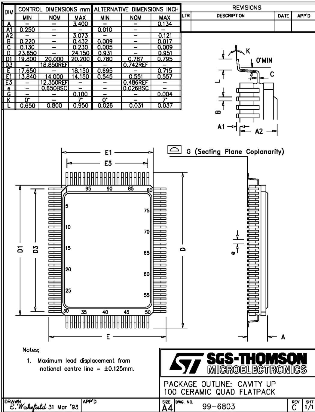
Figure 9.4 IMS T225E 100 pin cavity-up ceramic quad flat pack package dimensions
