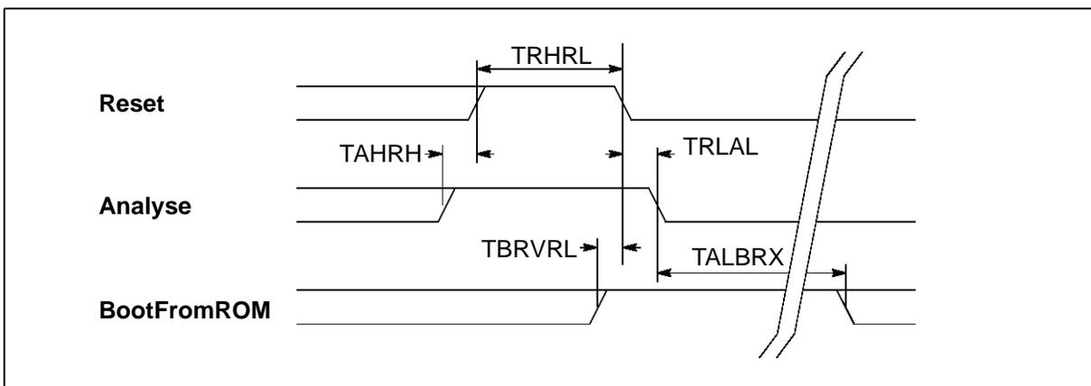
Figure 3.4 Transputer **Reset**, **Analyse** and **BootFromROM** timing
