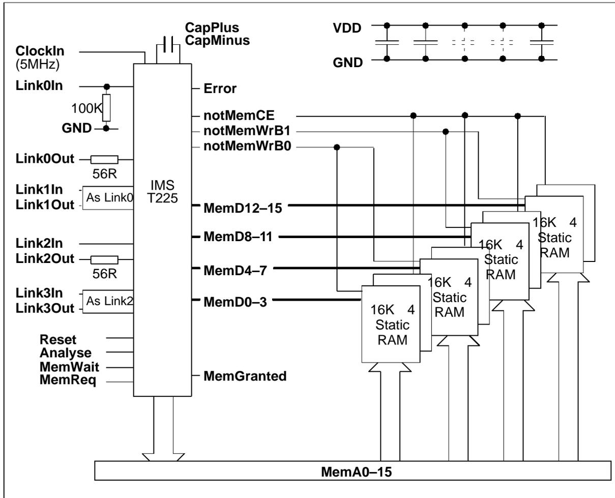
Figure 5.2 IMS T225E static RAM application
