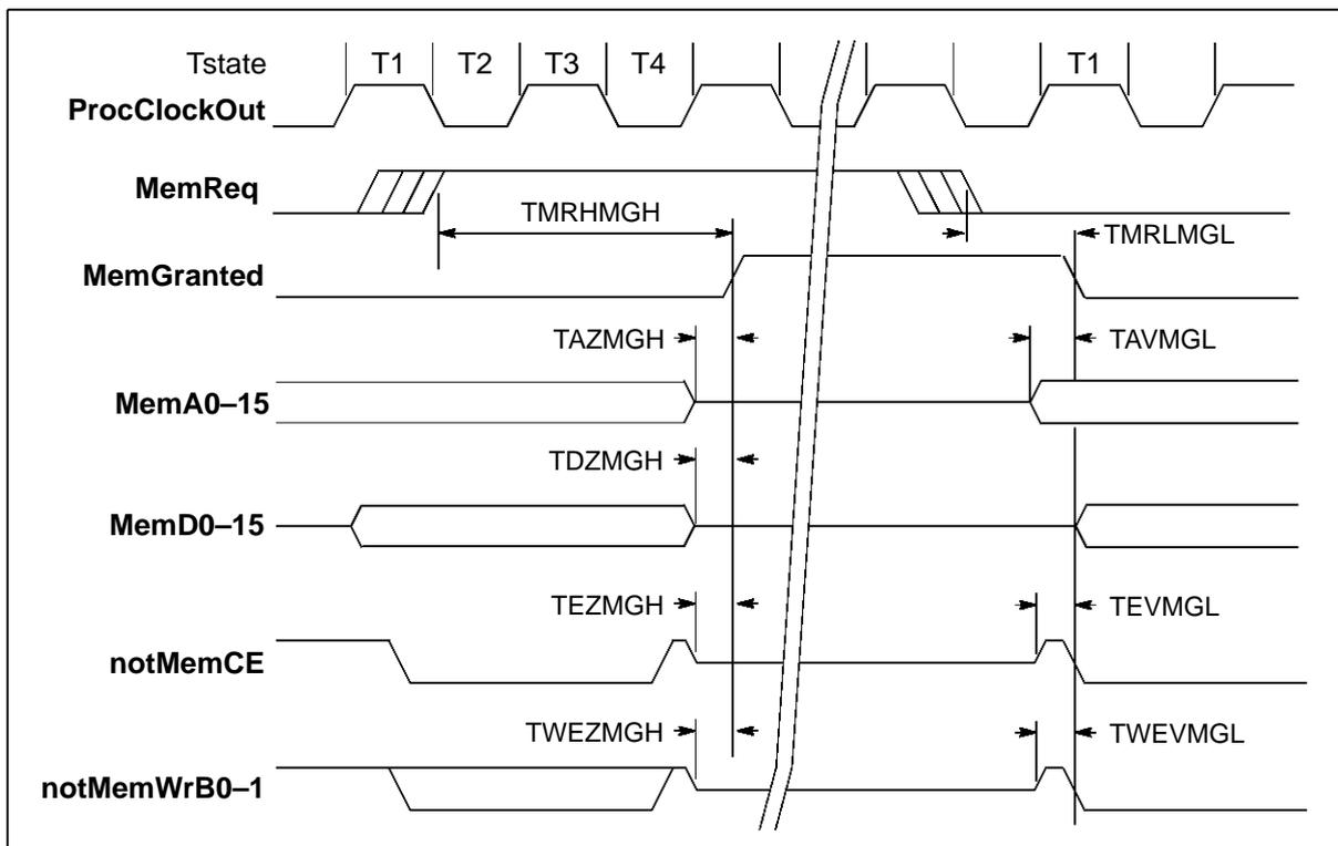
Figure 5.14 IMS T225E memory request timing
