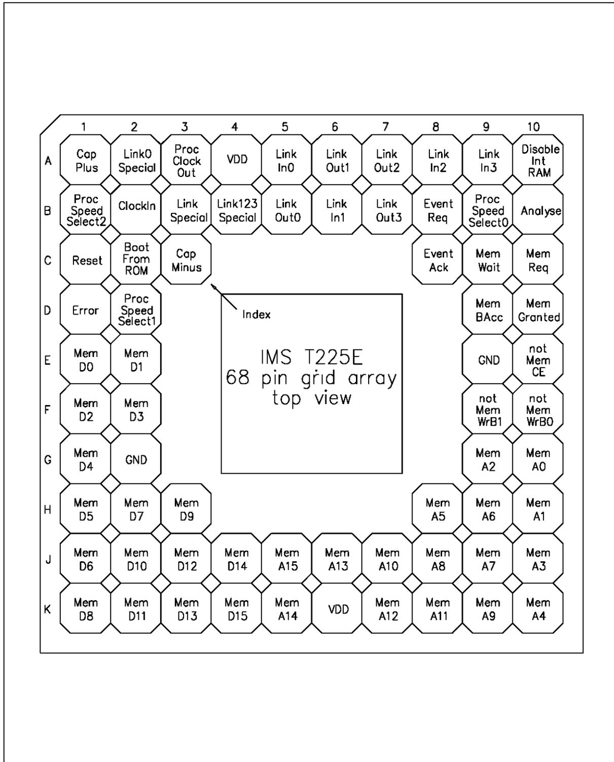
Figure 9.1 IMS T225E 68 pin grid array package pinout
