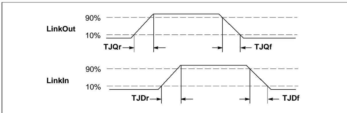
Figure 7.2 IMS T225E link timing
