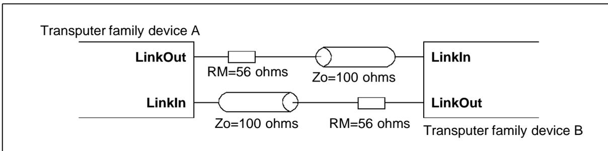
Figure 7.5 IMS T225E links connected by transmission line
