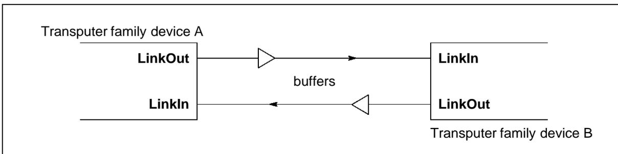
Figure 7.6 IMS T225E links connected by buffers
