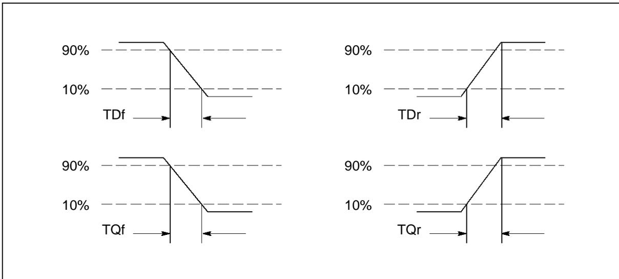
Figure 8.3 IMS T225E input and output edge timing
