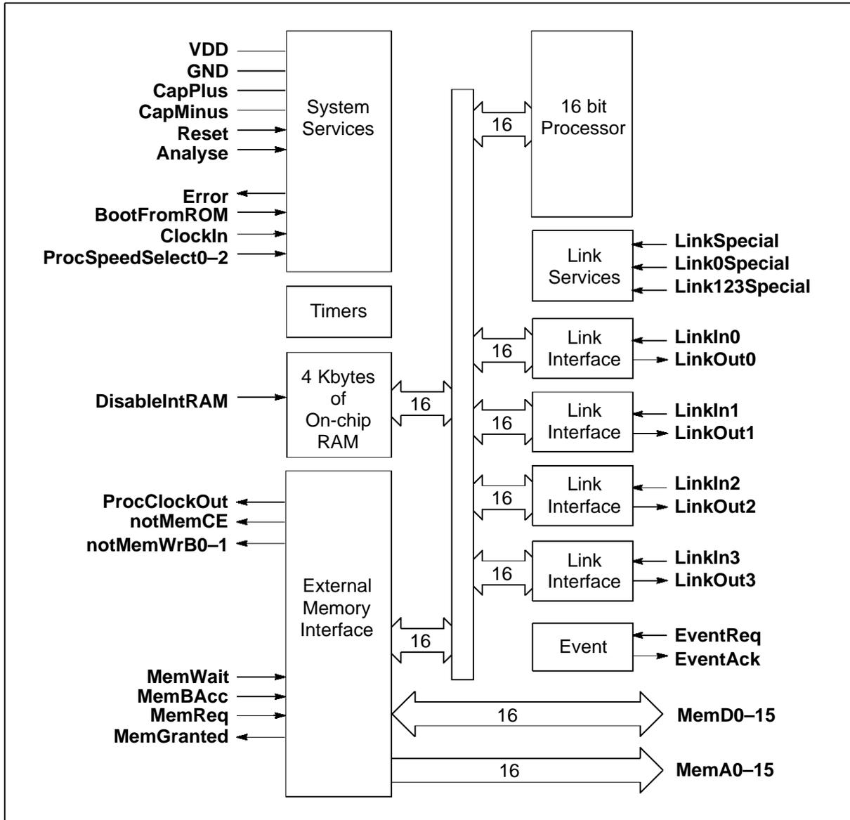
Figure 1.1 IMS T225E block diagram
