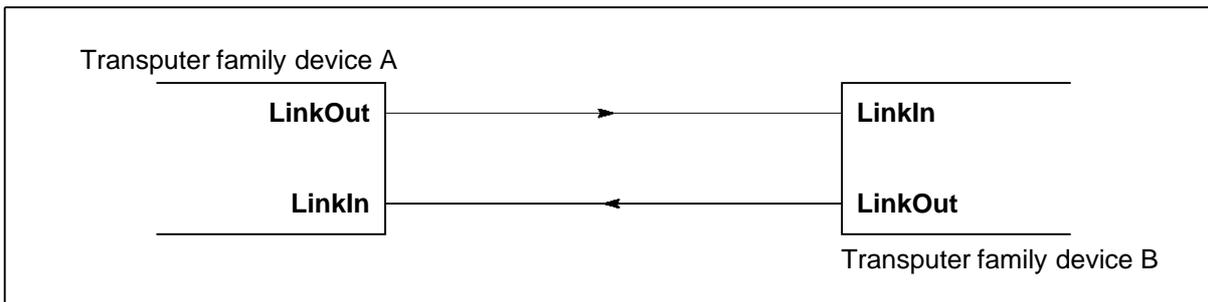
Figure 7.4 IMS T225E links directly connected
