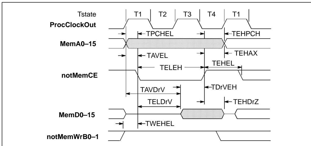
Figure 5.4 IMS T225E external read cycle
