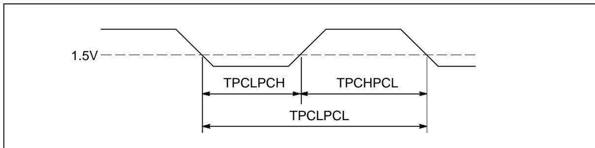
Figure 5.3 IMS T225E **ProcClockOut** timing
