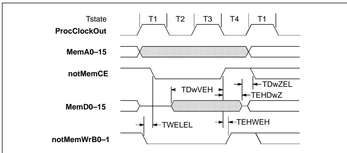
Figure 5.5 IMS T225E external write cycle
