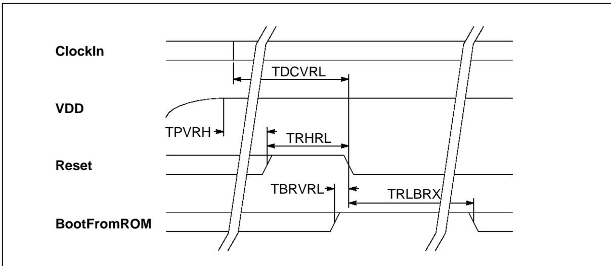
Figure 3.3 Transputer **Reset** timing with **Analyse** low
