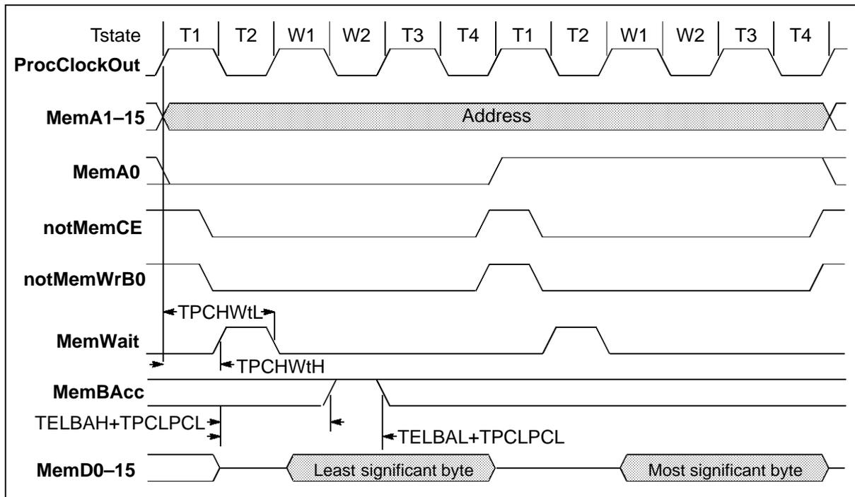
Figure 5.9 IMS T225E word write to byte wide memory with a single wait state
