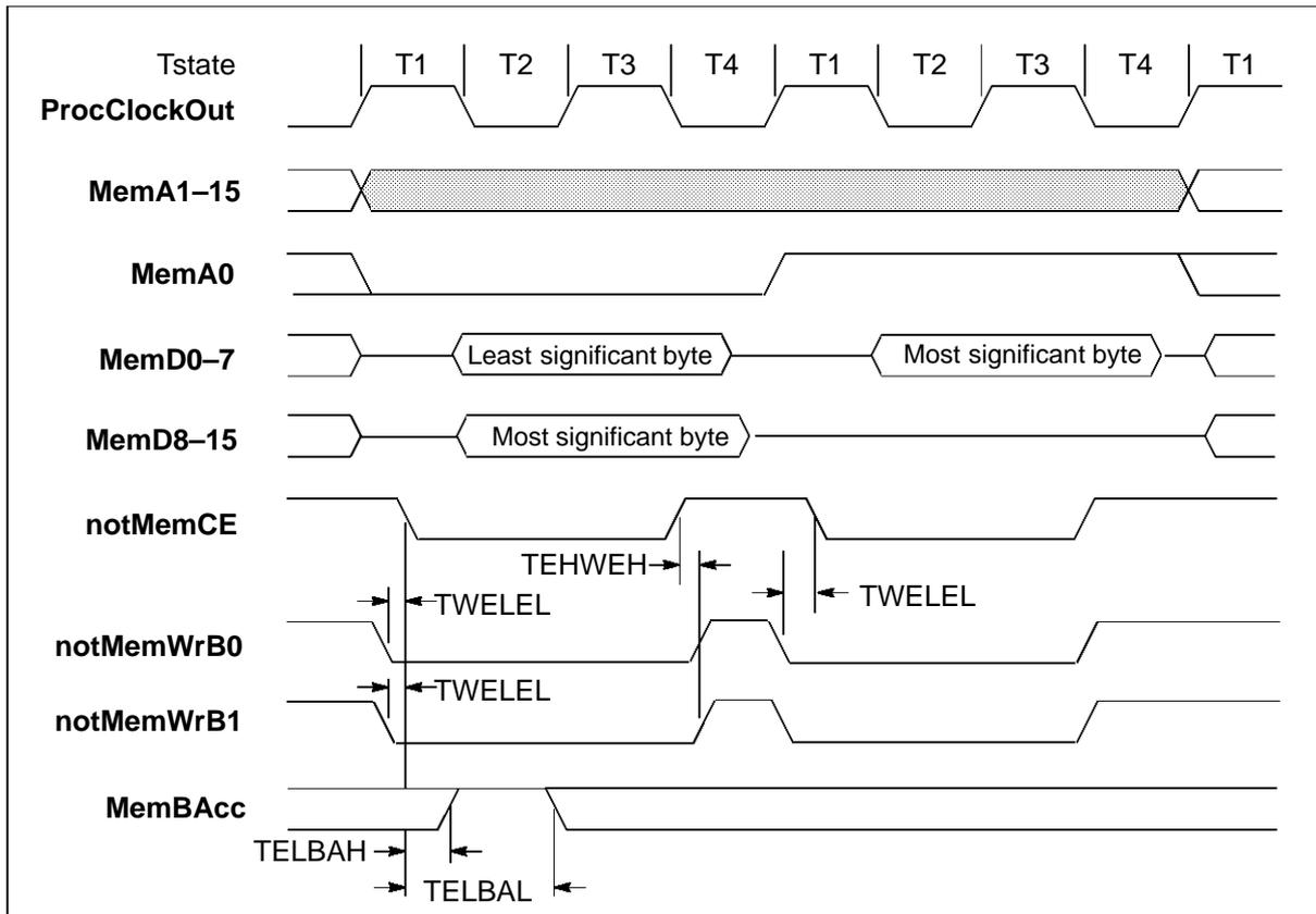
Figure 5.7 IMS T225E word write to byte-wide memory
