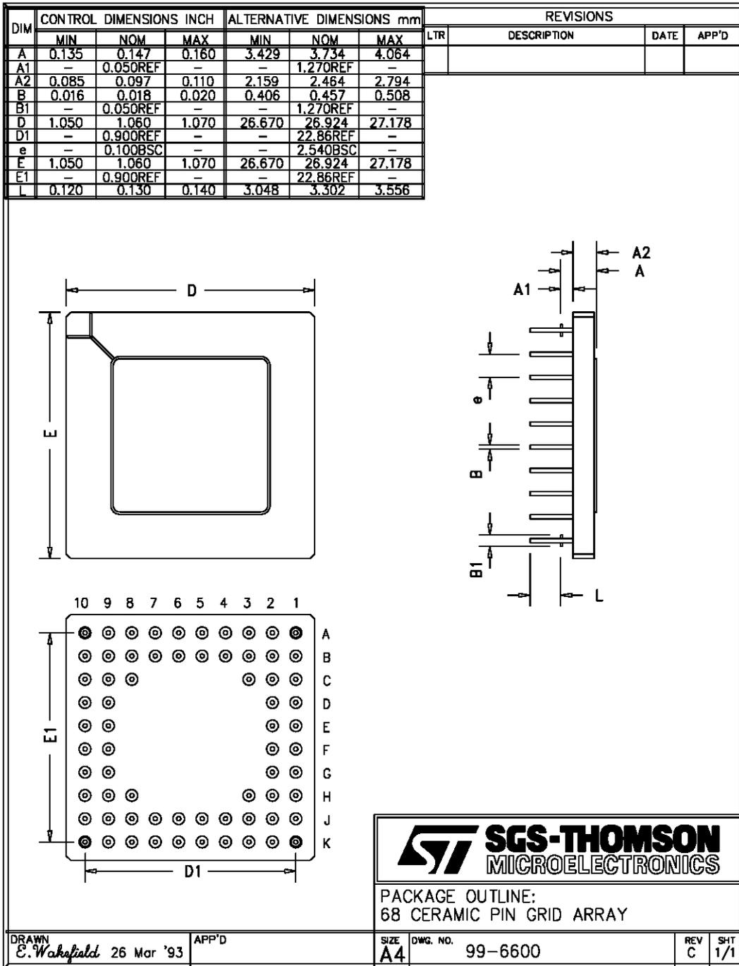
Figure 9.2 IMS T225E 68 pin grid array package dimensions
