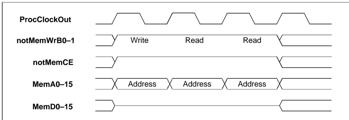
Figure 5.1 IMS T225E bus activity for 3 internal memory cycles
