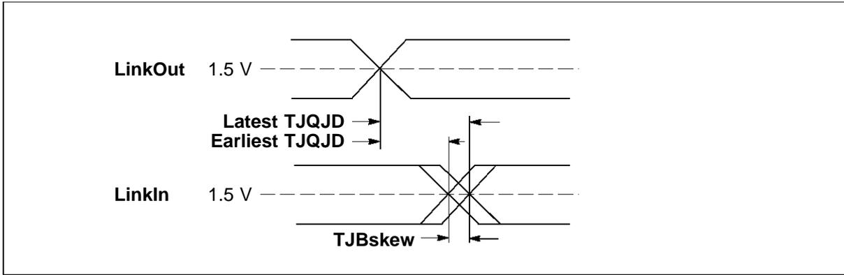
Figure 7.3 IMS T225E buffered link timing
