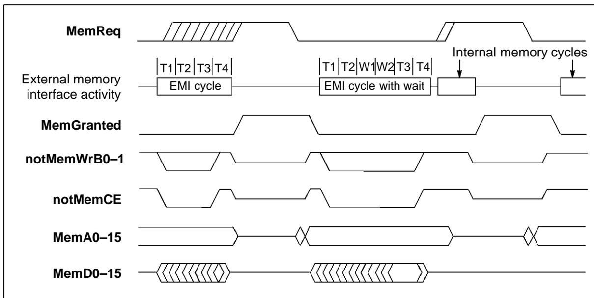
Figure 5.13 IMS T225E operation of **MemReq** and **MemGranted** with external and internal memory cycles
