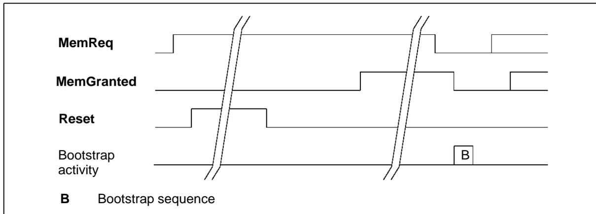
Figure 5.12 IMS T225E DMA sequence at reset
