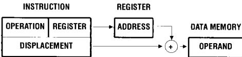
THE OPERAND VALUE IS THE CONTENTS OF THE LOCATION WHOSE ADDRESS IS THE ADDRESS IN THE INSTRUCTION, OFFSET BY THE CONTENTS OF THE REGISTER.
