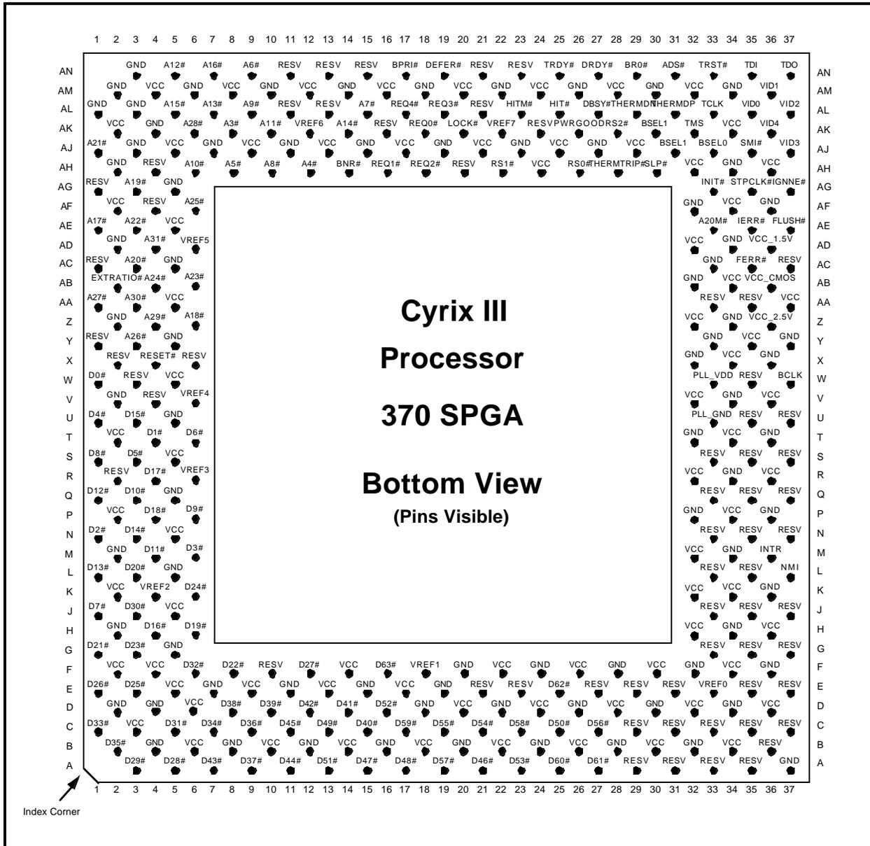
Figure 5-1. Bottom View 370-Pin SPGA Package Pin Assignments
