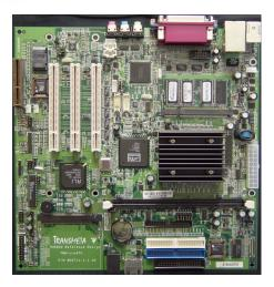
The TM5800 MicroATX motherboard is a high-performance multimedia platform reference design based on the Transmeta Crusoe<sup>™</sup> model TM5800 microprocessor. The MicroATX reference design motherboard comes with schematics, design guides, processor specifications, and everything else needed to jump-start new product design efforts with a fully-functional and fully-documented desktop and mobile PC system design.
